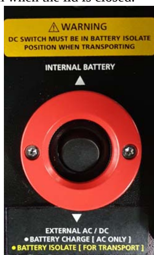
Figure 3.1 Battery select switch
