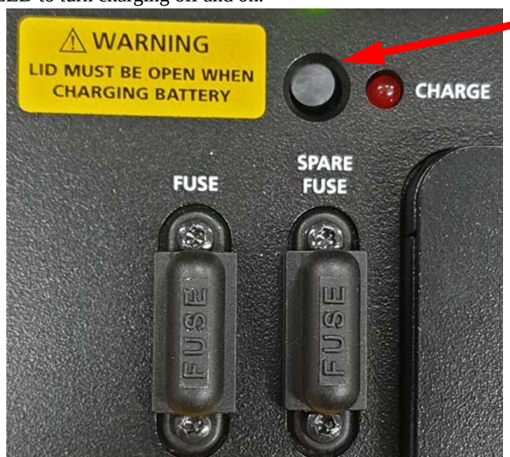
Figure 3.2 Recessed charge button
