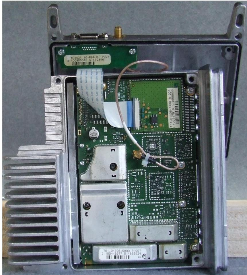
Photograph 11: Power Amplifier PCB – Top
