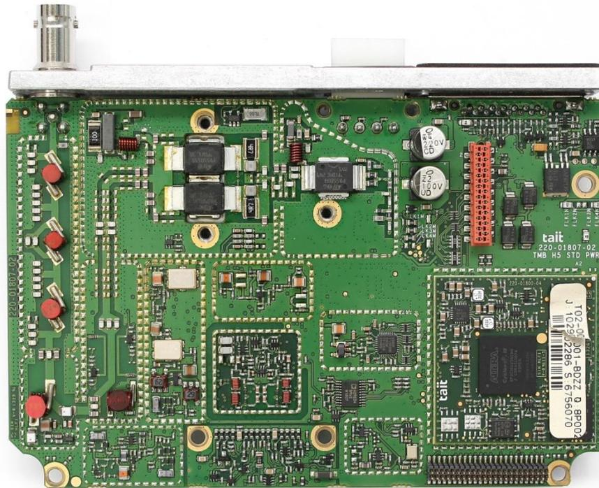
Photograph 12: Power Amplifier PCB – Top, cans off
