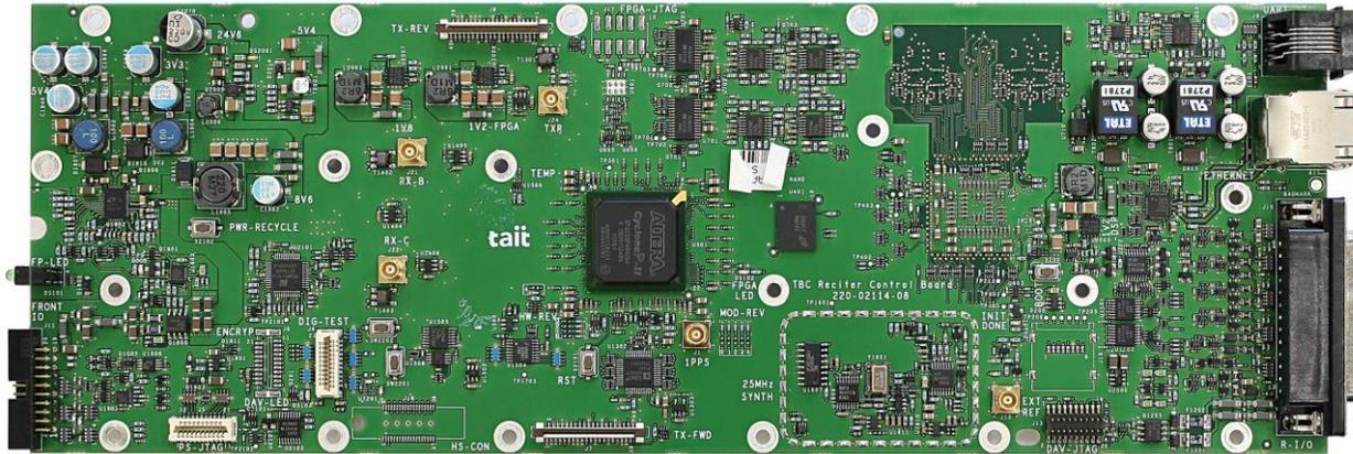
Photograph 15: Reciter Control Board (RCB) – Top (can off)
