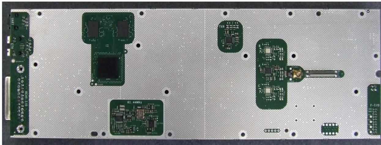
Photograph 16: Reciter Control Board (RCB) – Bottom
