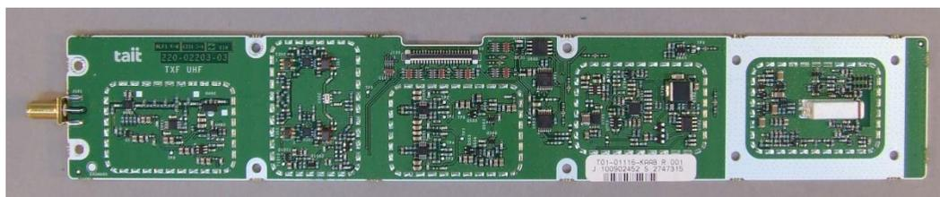
Photograph 21: Transmit Forward Power Board (TXF) – Top (cans off)
