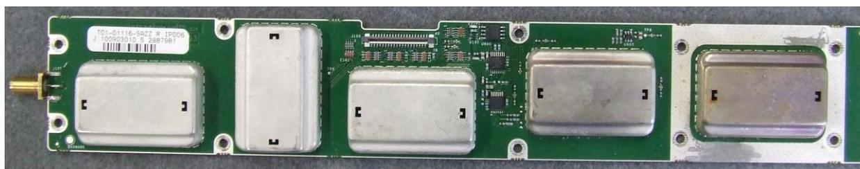
Photograph 20: Transmit Forward Power Board (TXF) – Top
