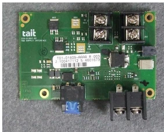
Photograph 09: Supply Interface PCB - Top
