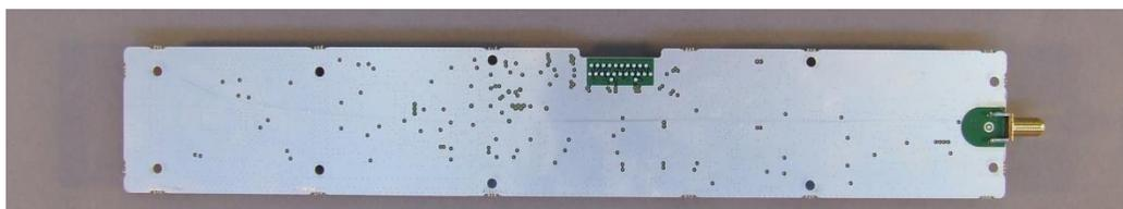
Photograph 22: Transmit Forward Power Board (TXF) – Bottom
