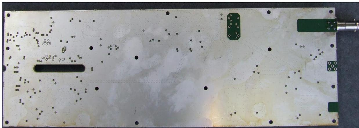
Photograph 19: Receiver Board (RXB) – Bottom
