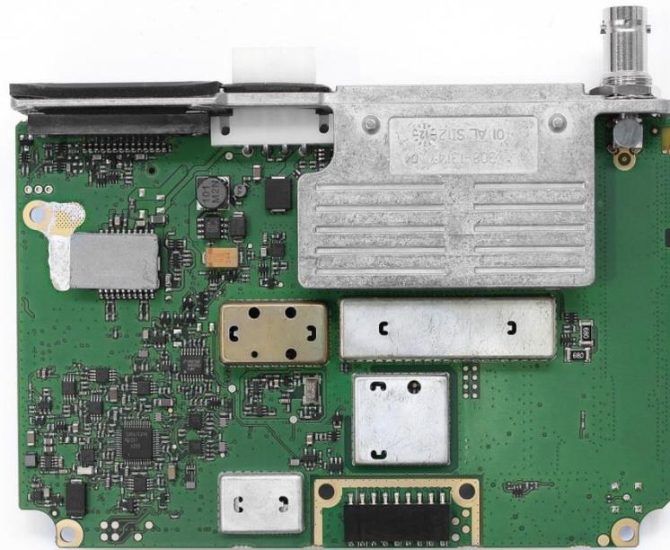
Photograph 13: Power Amplifier PCB – Bottom
