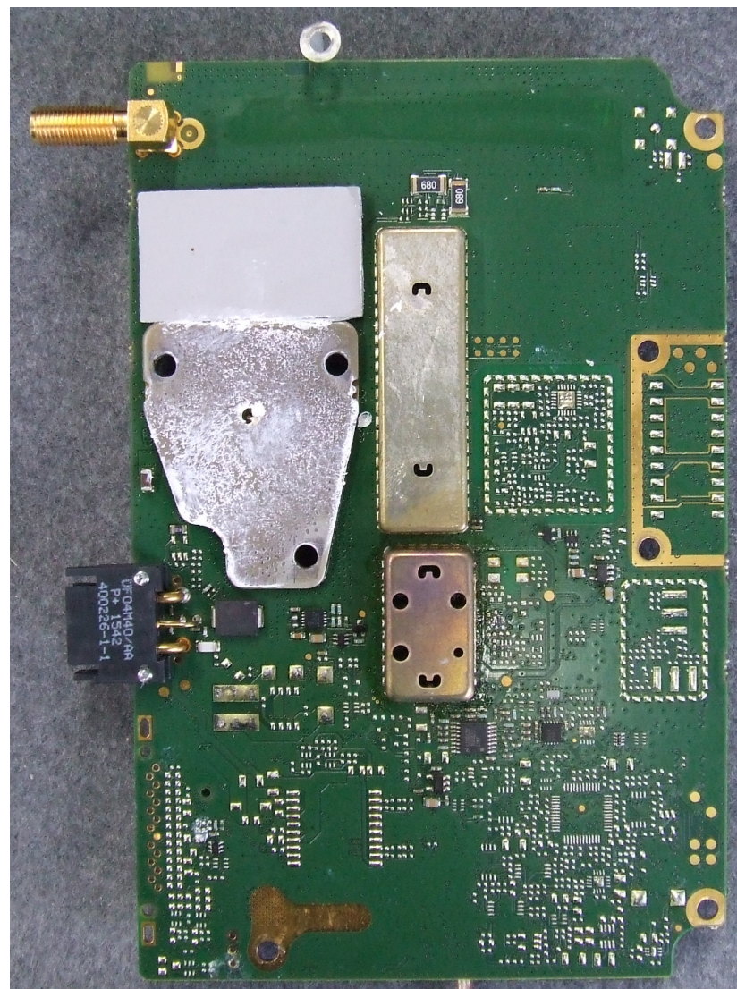
Photograph 09: Power Amplifier PCB – Bottom
