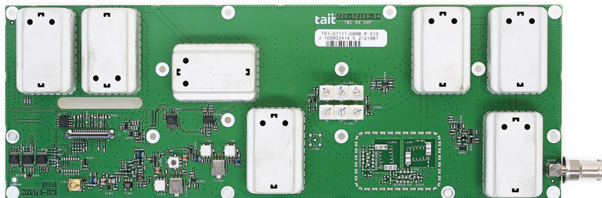
Photograph 13: Receiver Board (RXB) – Top
