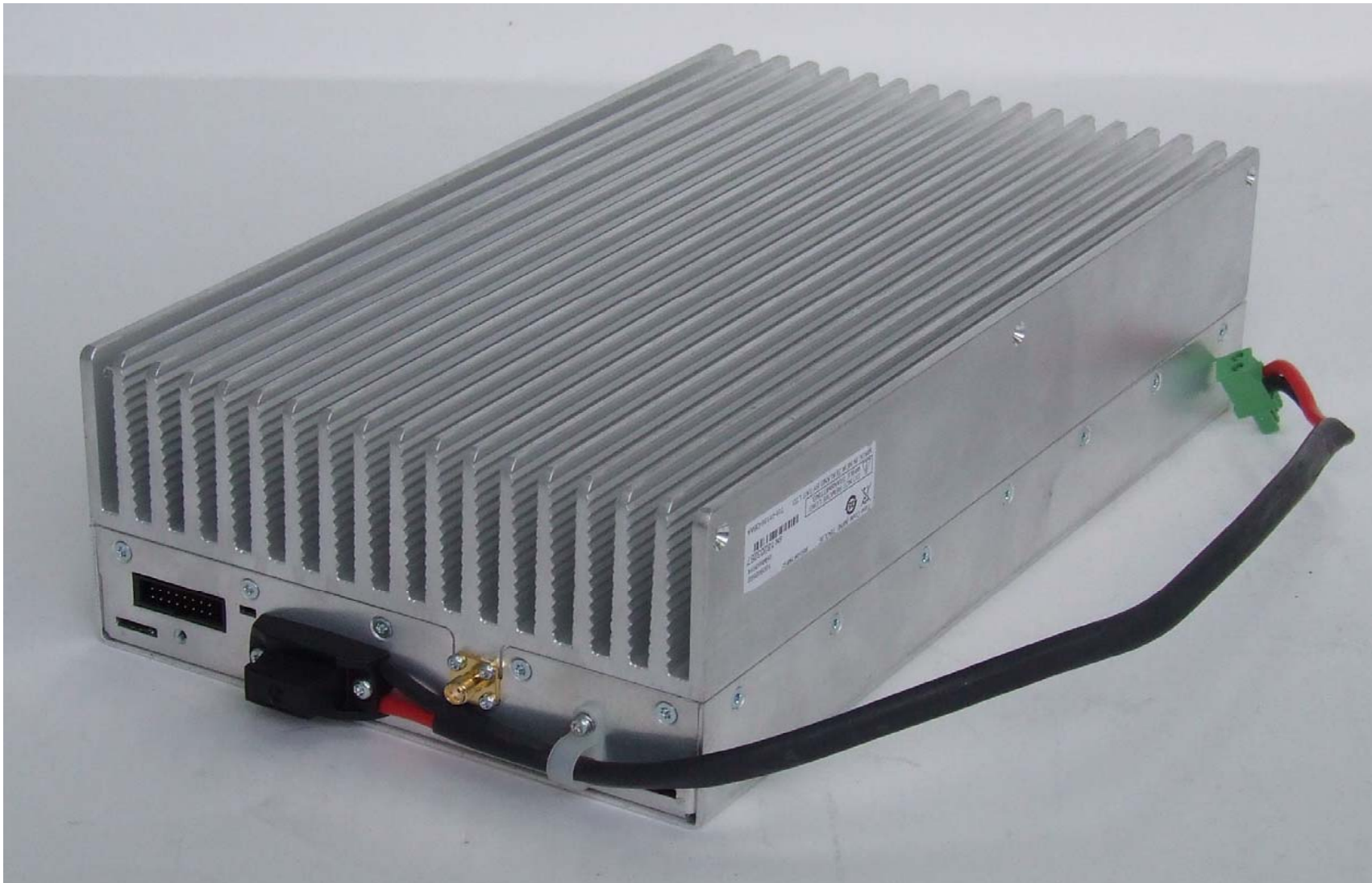
Photograph 05: 100W PA module – Product view
