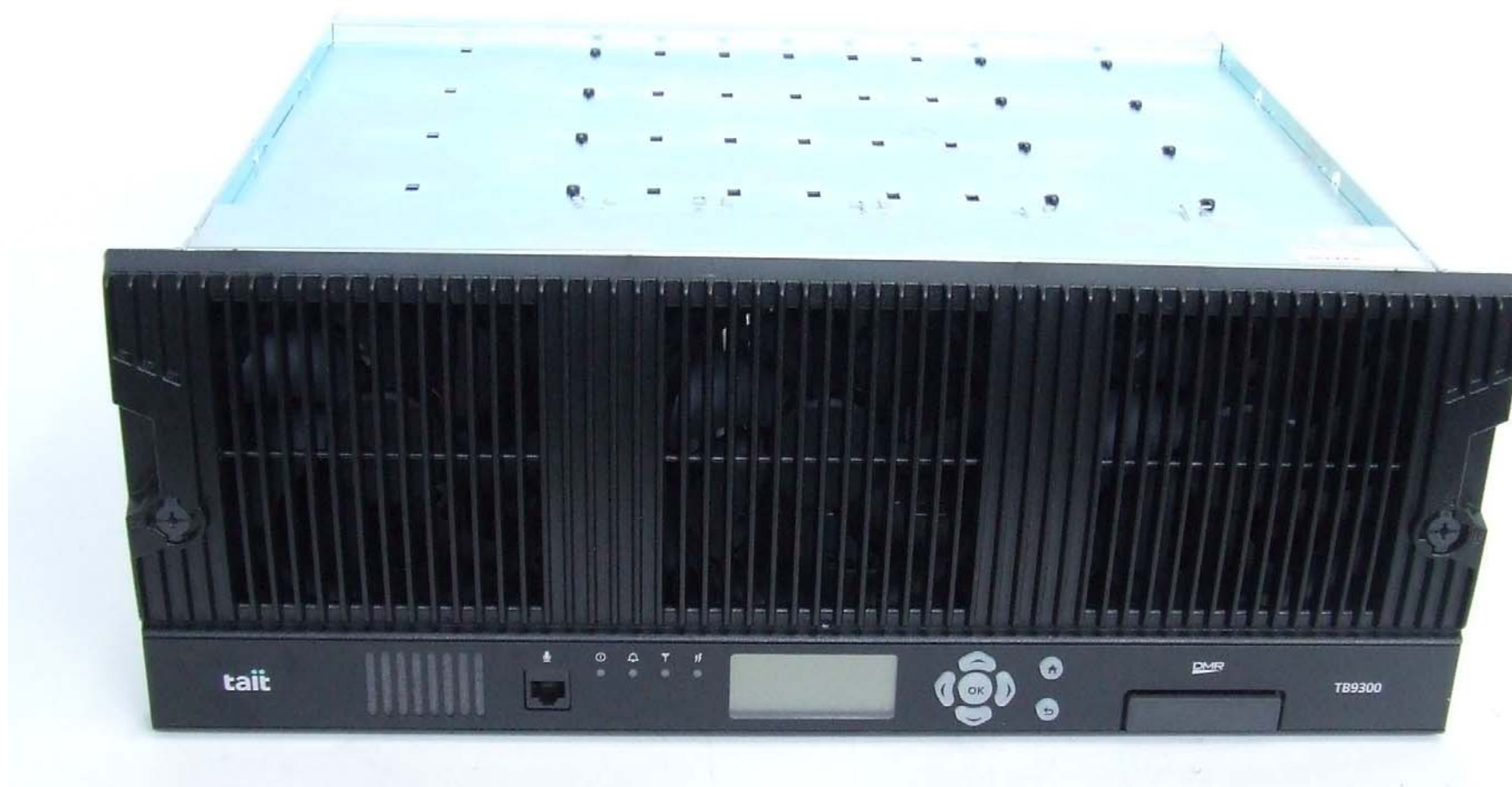
Photograph 02: 100W System – Front panel
