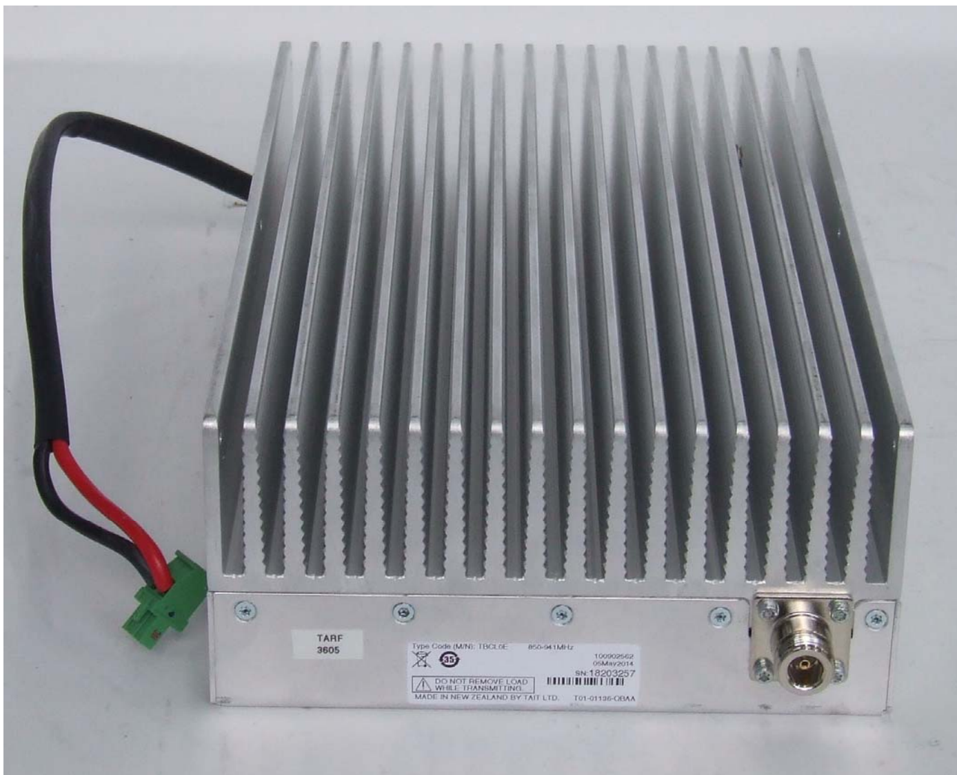
Photograph 07: 100W PA module – Rear panel
