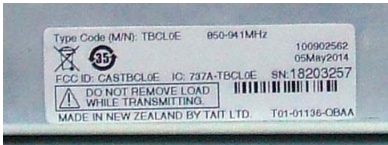
Photograph 03: 100W PA module (850→941MHz) – Compliance label
