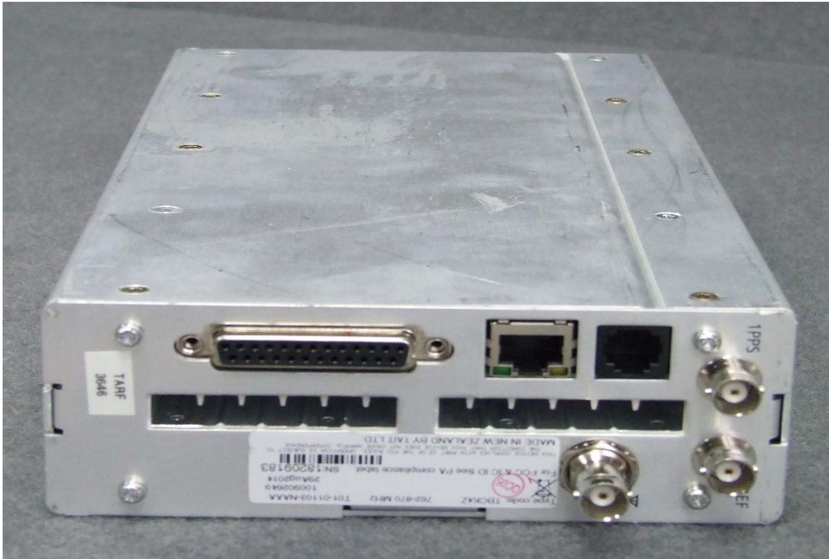
Photograph 09: Reciter module (762-870MHz) – Rear panel
