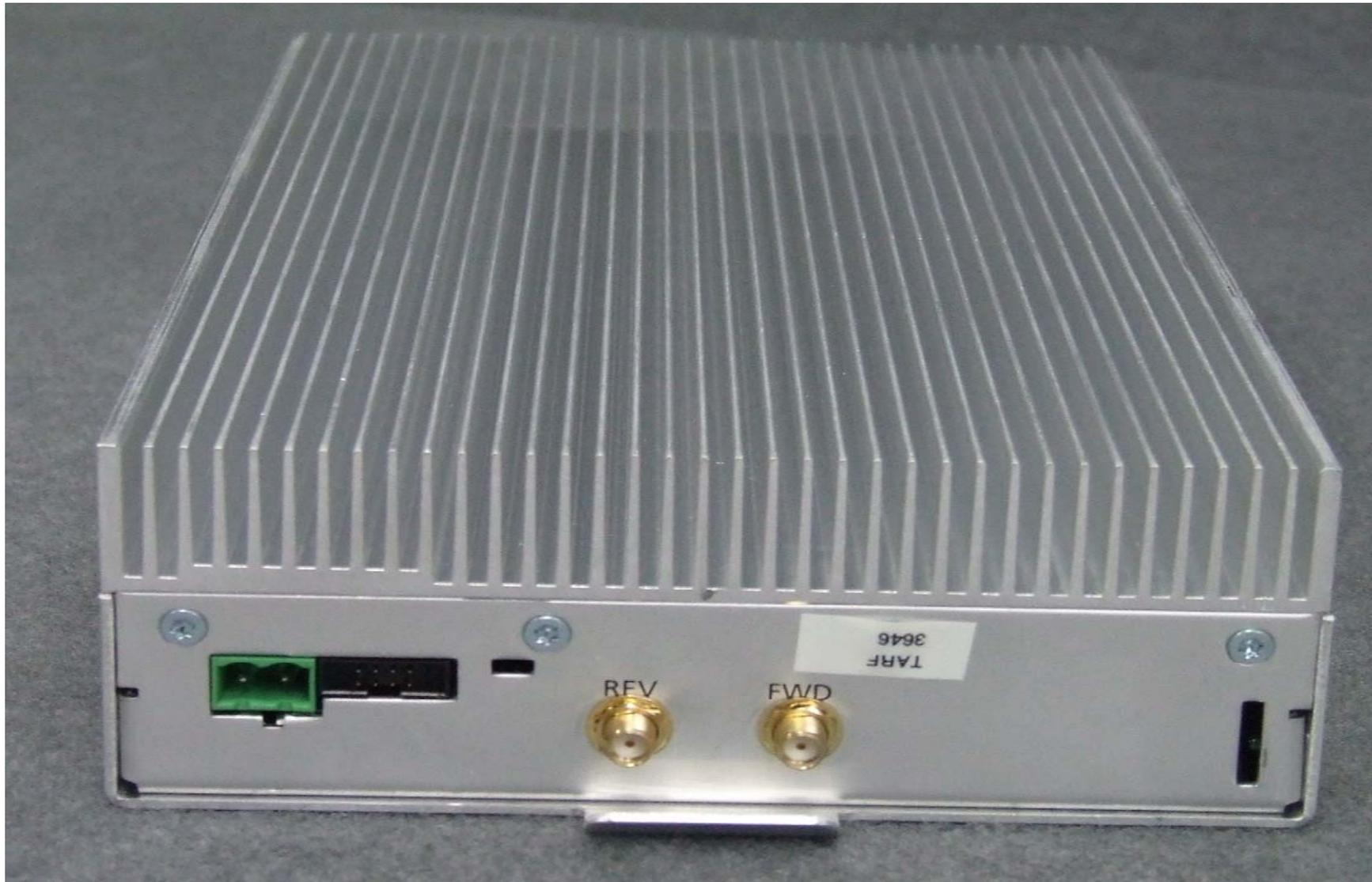
Photograph 06: 50W PA module – Front panel
