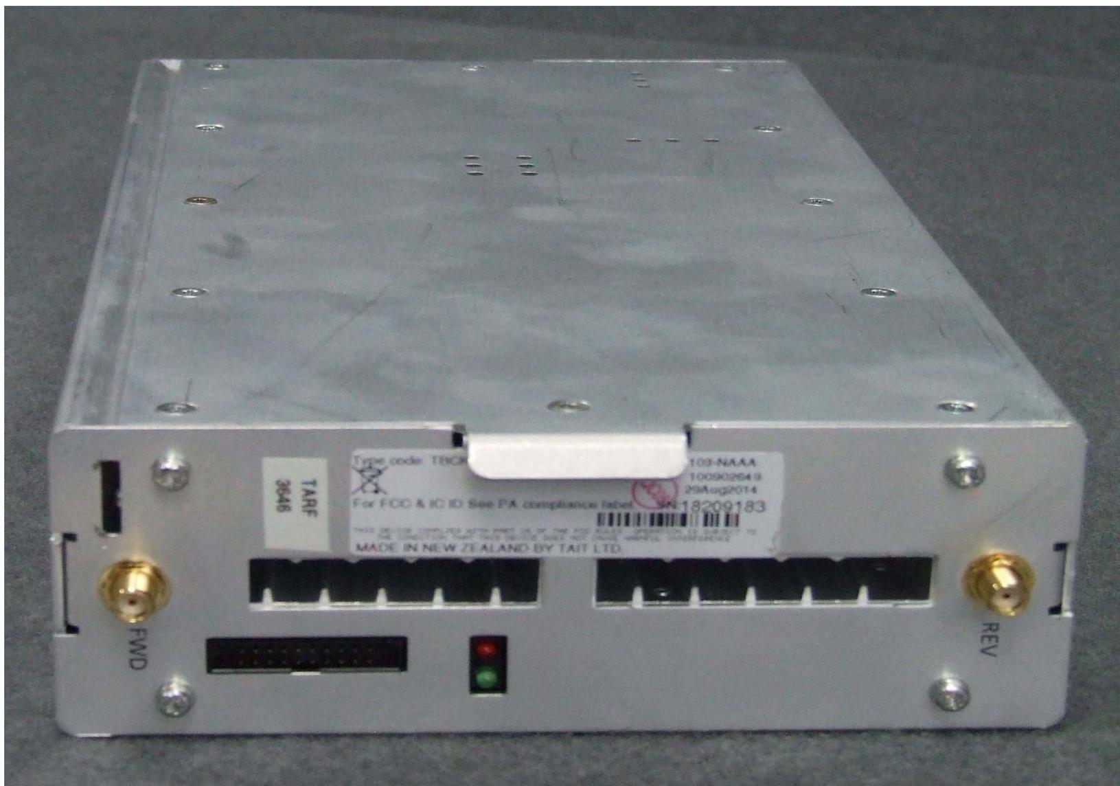
Photograph 08: Reciter module (762-870MHz) – Front panel
