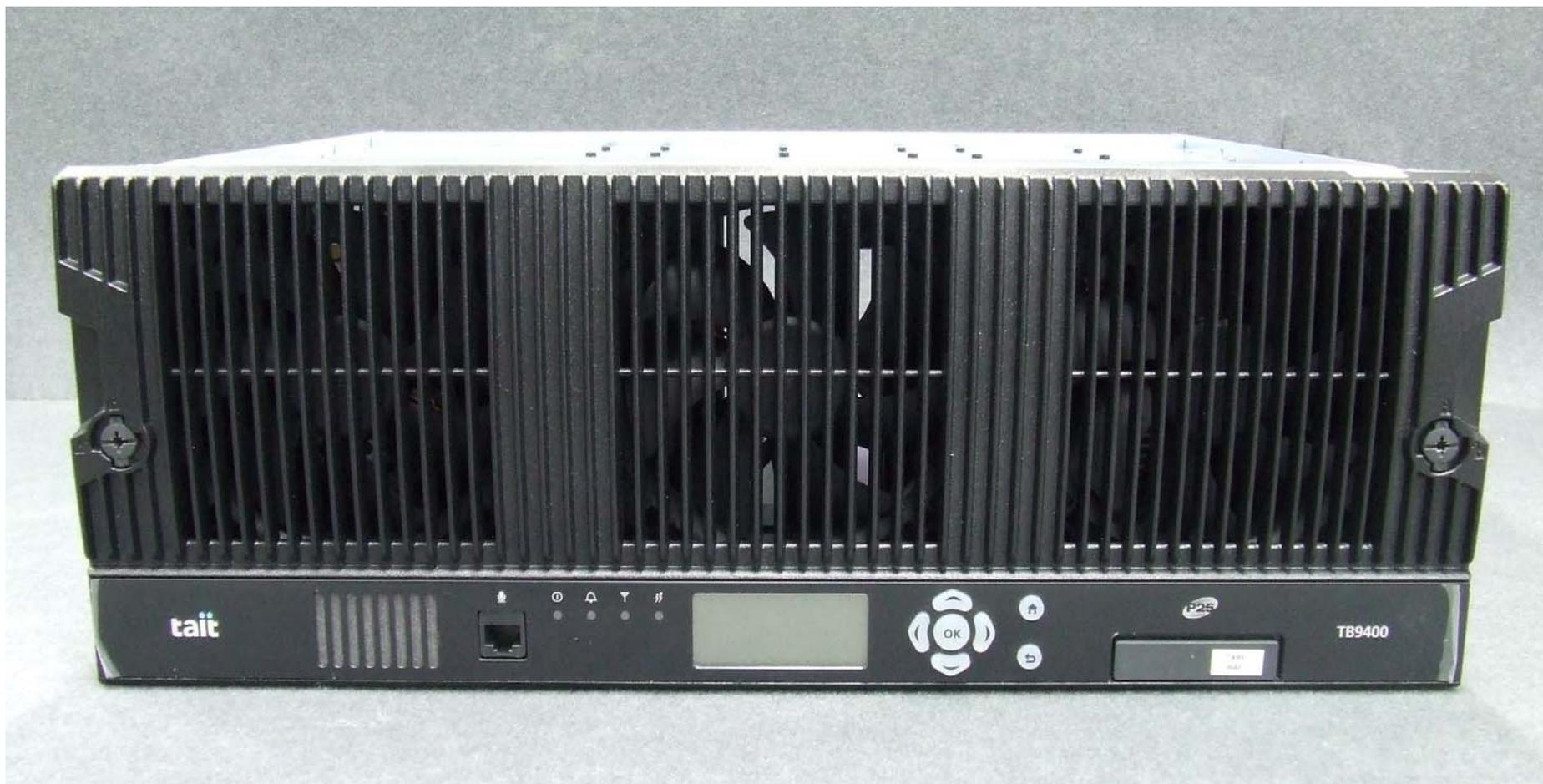
Photograph 02: 50W System – Front panel
