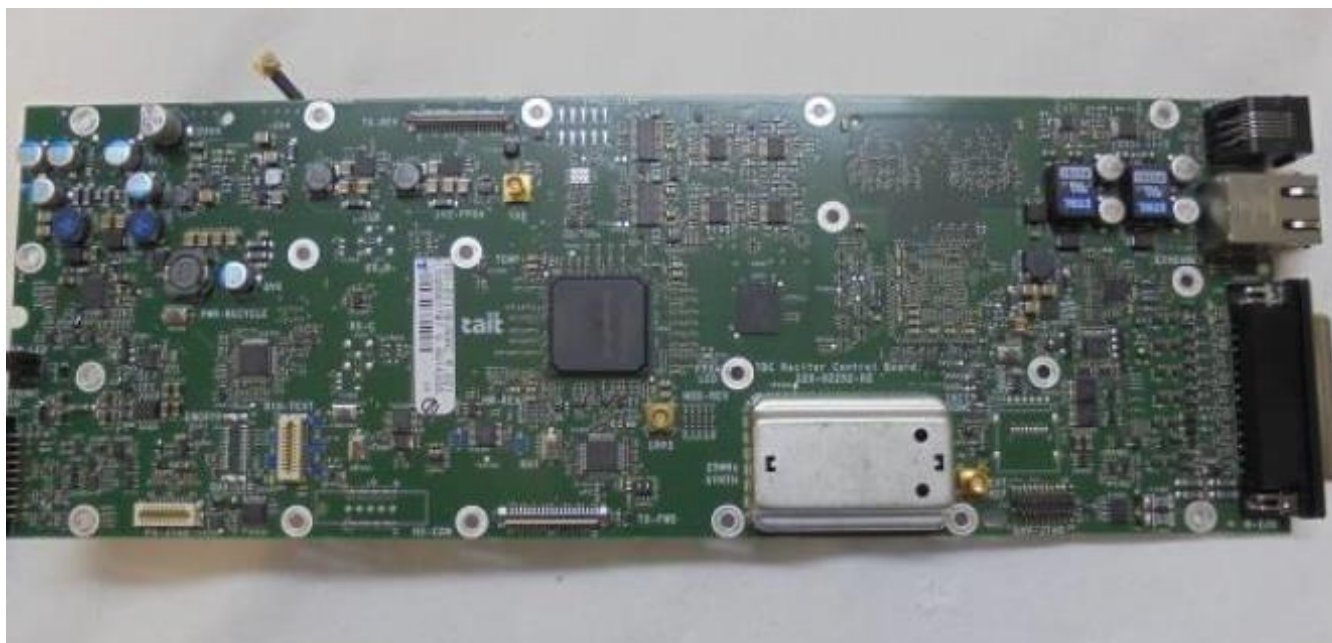
Photograph 06: Reciter Control PCB – Top (with shields)
