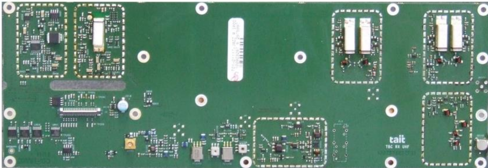
Photograph 04: Reciter Receiver PCB – Top (without shields)
