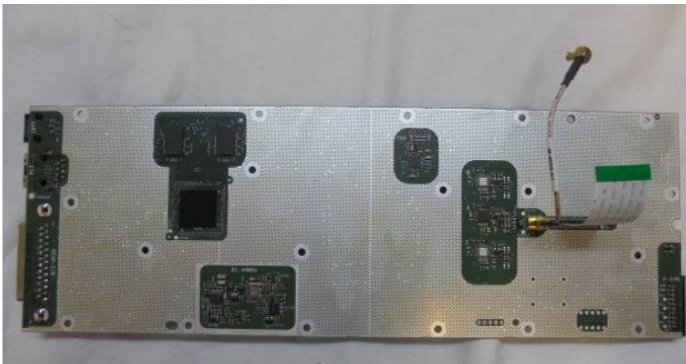
Photograph 08: Reciter Control PCB – Bottom
