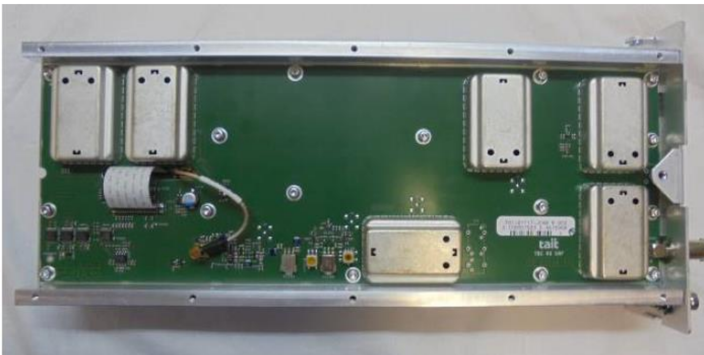
Photograph 01: Reciter module – Internal (Receiver PCB side)
