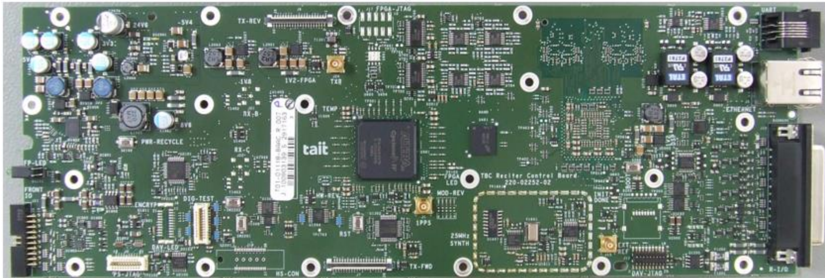
Photograph 07: Reciter Control PCB – Top (without shields)
