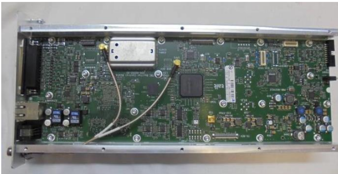
Photograph 02: Reciter module – Internal (Control PCB side)
