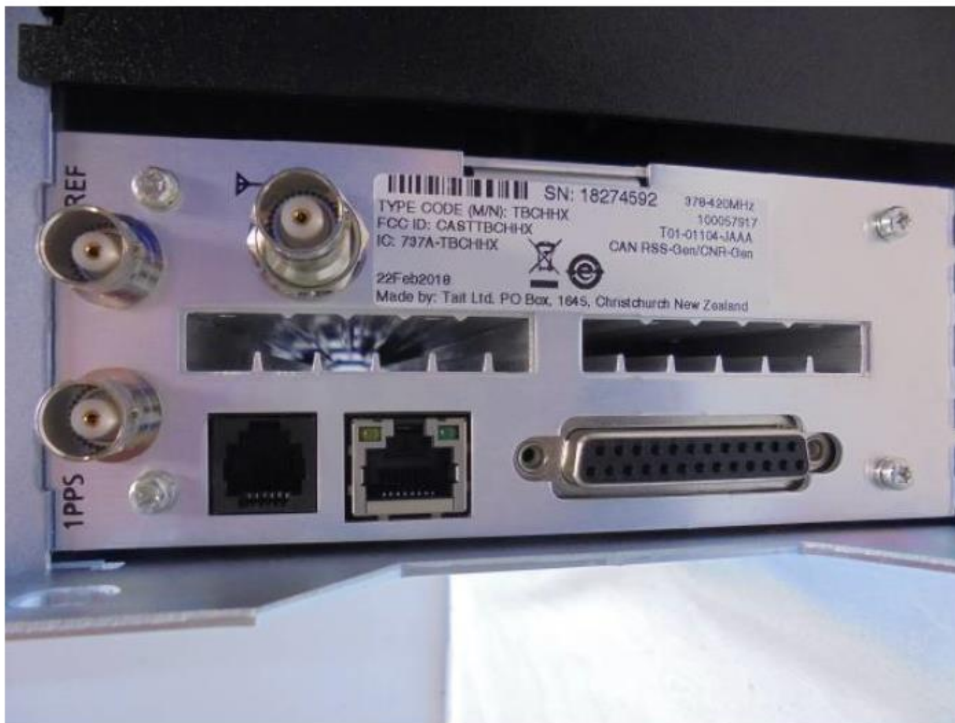
Photograph 07: Reciter module – Rear panel
