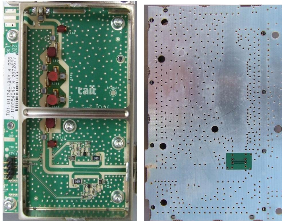
Photograph 29 & 30: Power Amplifier LPF PCB – Top & Bottom
