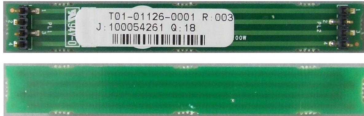
Photograph 27 & 28: Power Amplifier Interconnect PCB – Top & Bottom
