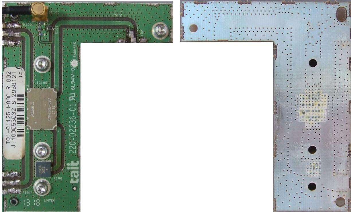
Photograph 25 & 26: Power Amplifier Combiner PCB – Top & Bottom
