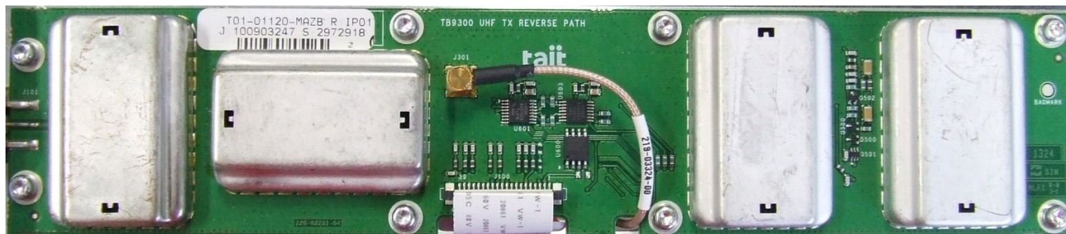
Photograph 12: Reciter TXR PCB – Top
