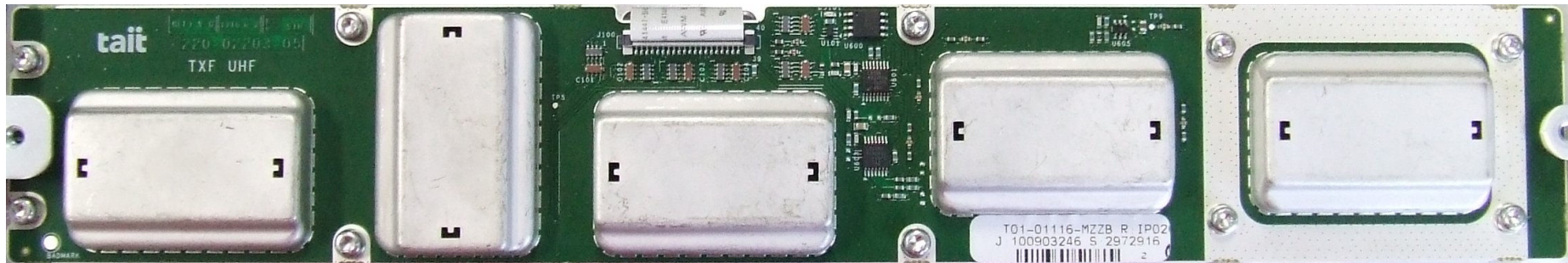
Photograph 09: Reciter TXF PCB - Top
