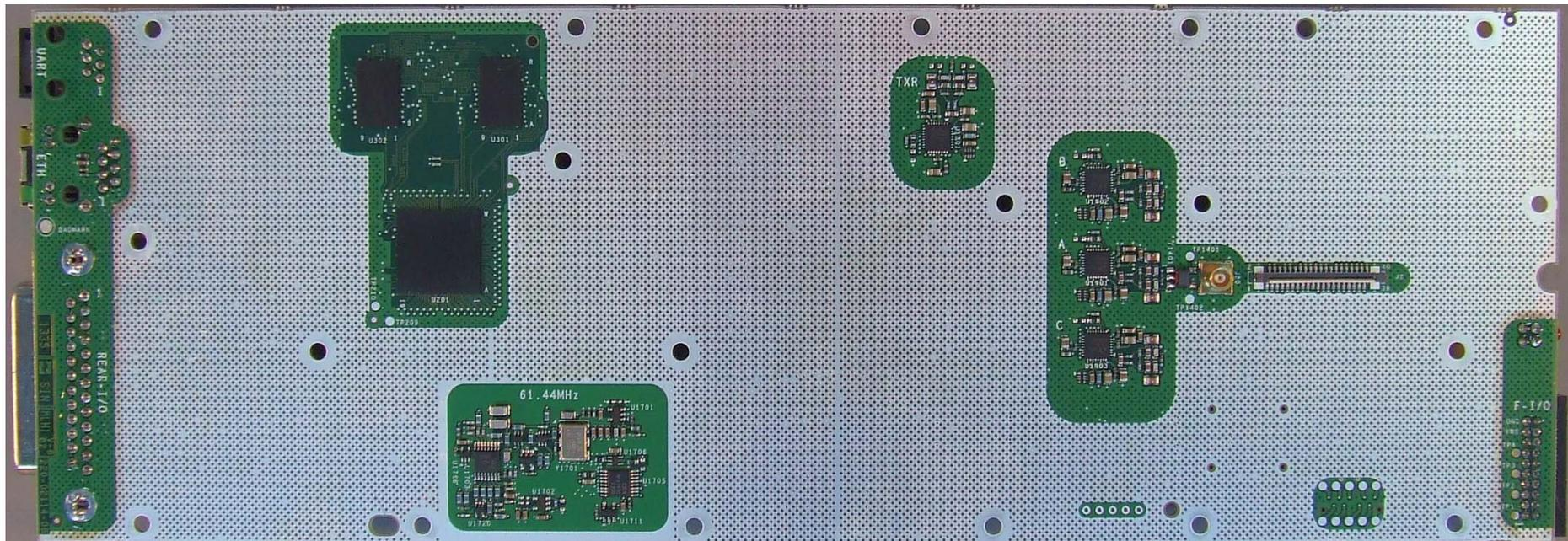
Photograph 14: Reciter Control PCB – Bottom
