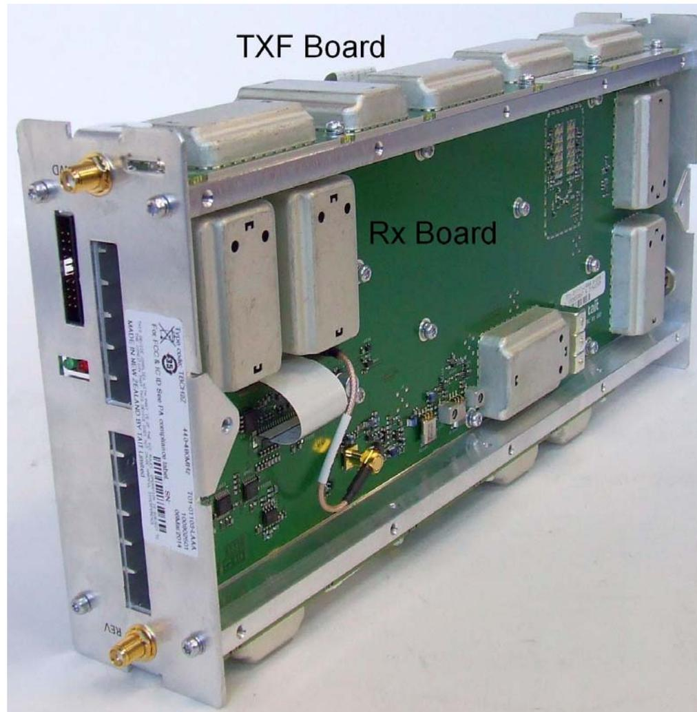
Photograph 10: Reciter module – Internal (Receiver PCB side)
