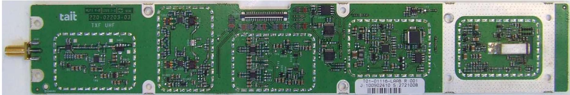
Photograph 19: Reciter TXF PCB – Top (without shields)
