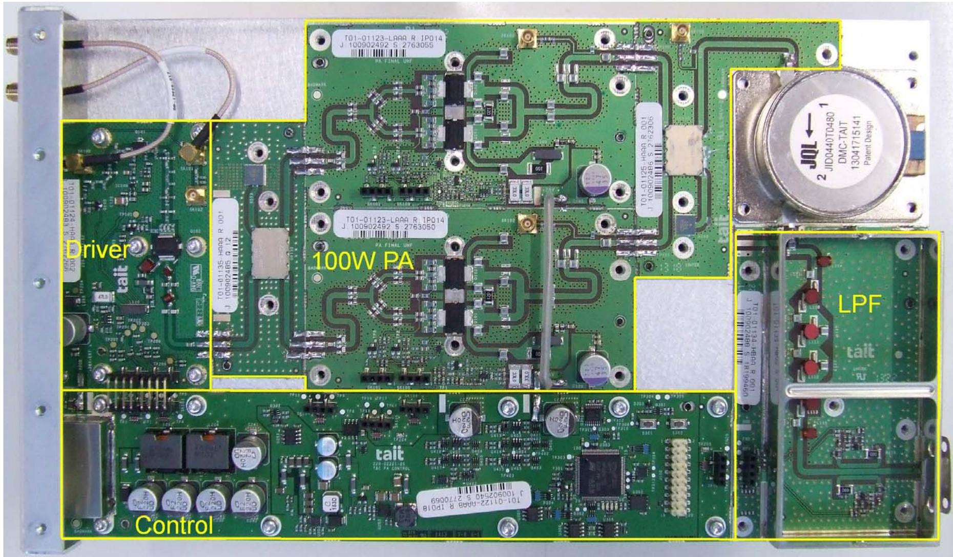
Photograph 01: 100W PA module – Internal view
