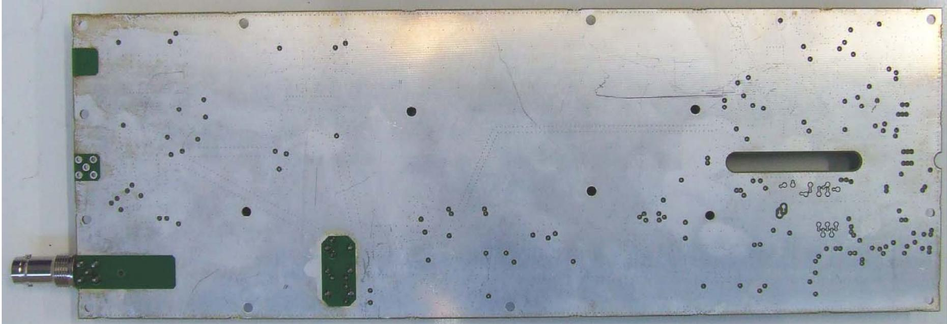
Photograph 17: Reciter Receiver PCB – Bottom
