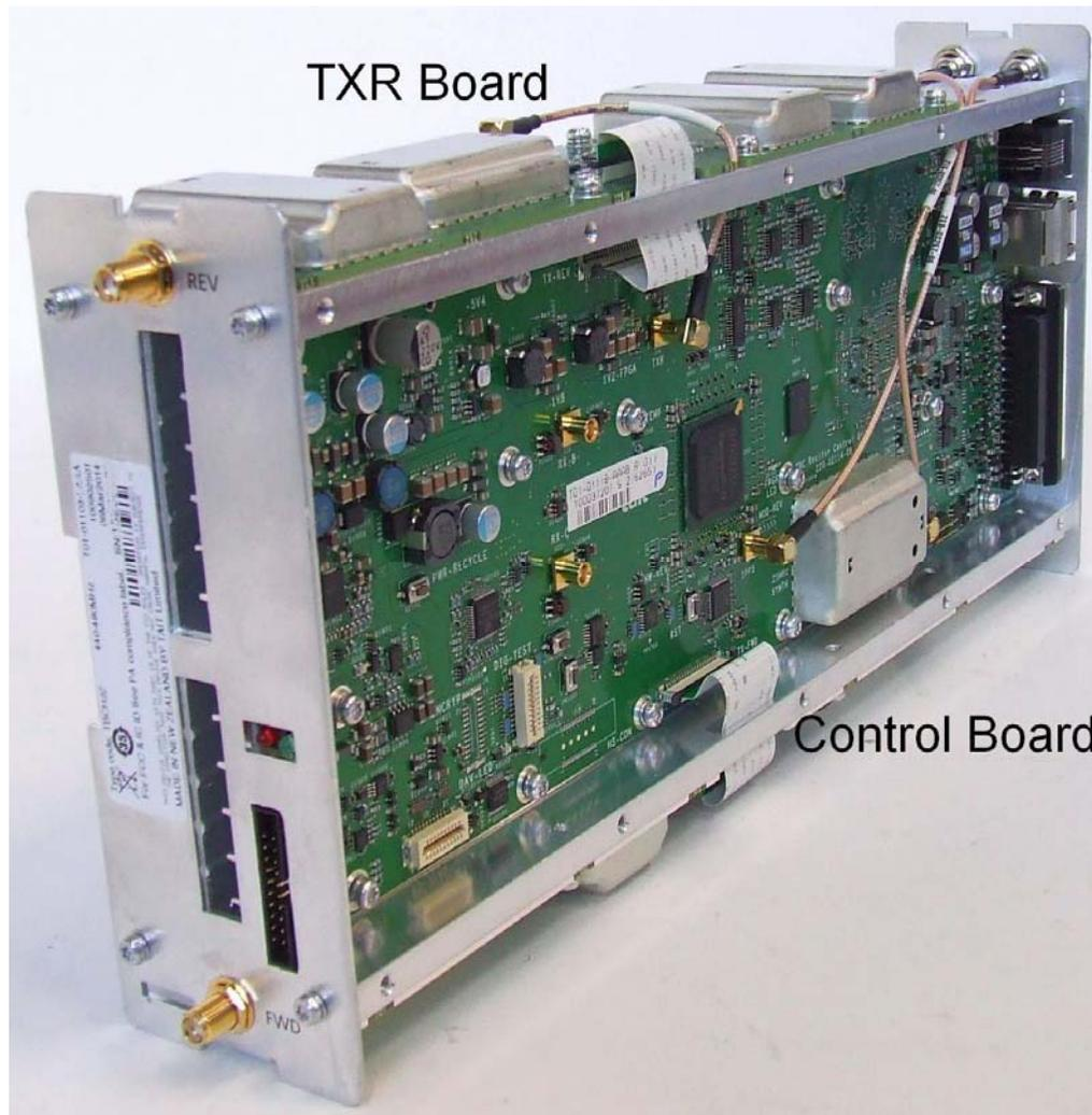
Photograph 11: Reciter module – Internal (Control PCB side)
