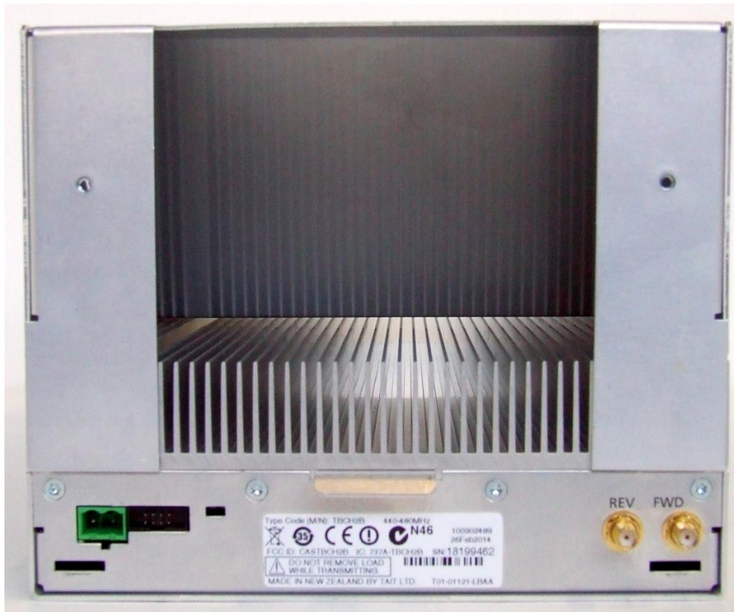
Photograph 07: PA module – Front panel
