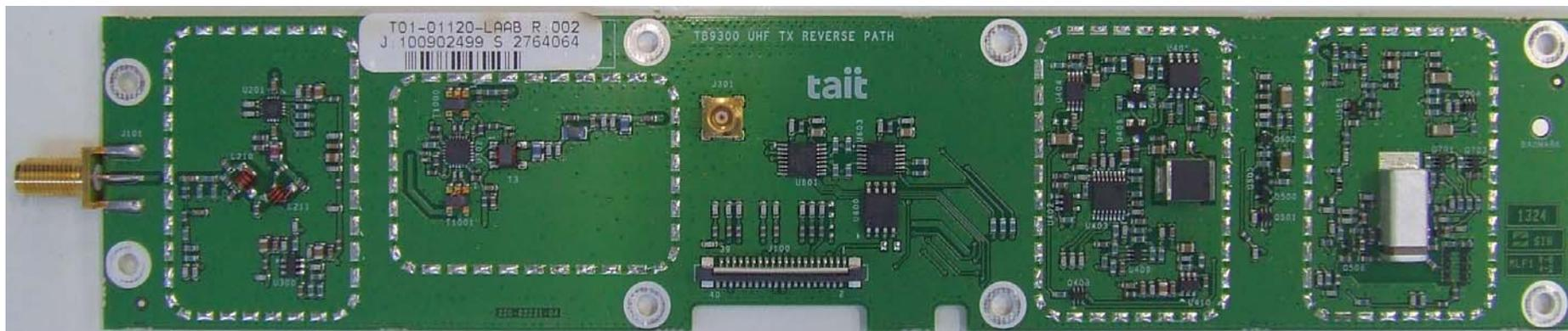
Photograph 22: Reciter TXR PCB – Top (without shields)
