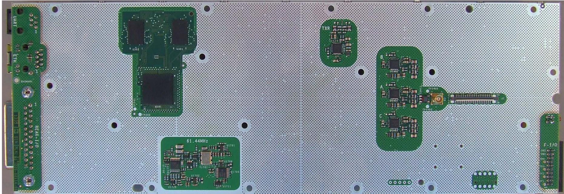
Photograph 14: Reciter Control PCB – Bottom
