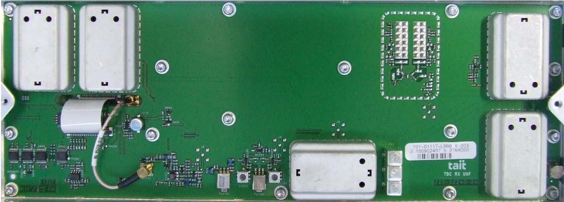
Photograph 15: Reciter Receiver PCB – Top (with shields)
