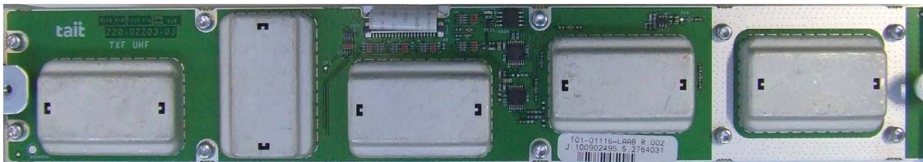
Photograph 18: Reciter TXF PCB – Top (with shields)
