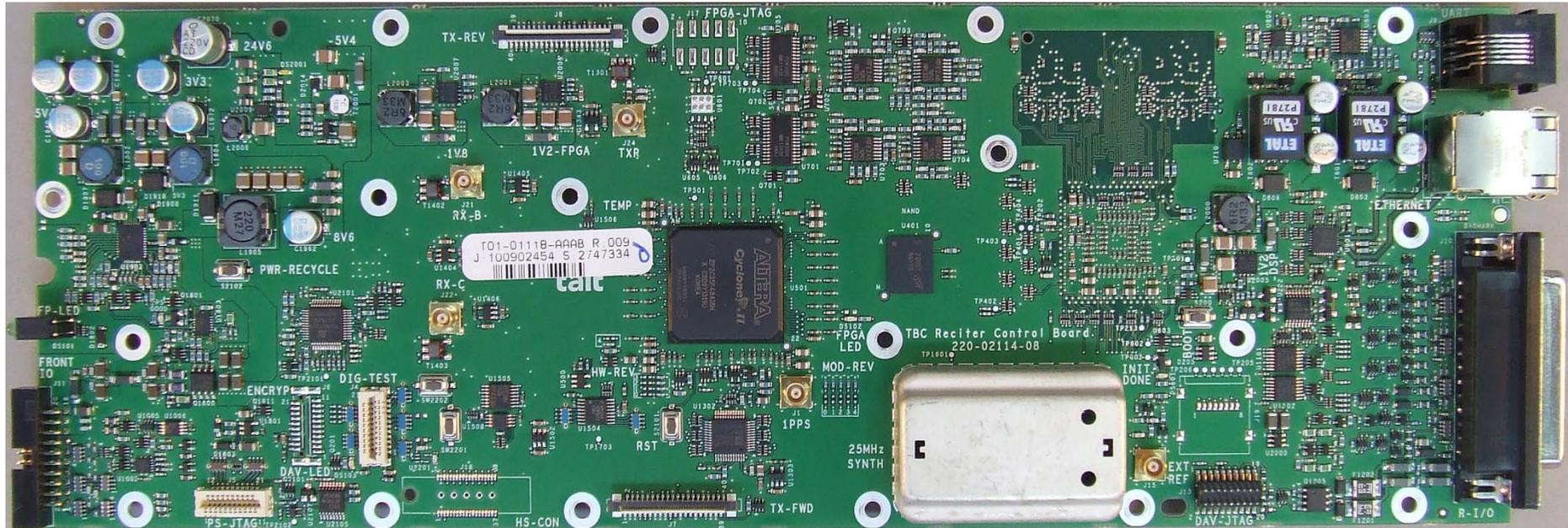
Photograph 12: Reciter Control PCB – Top (with shields)
