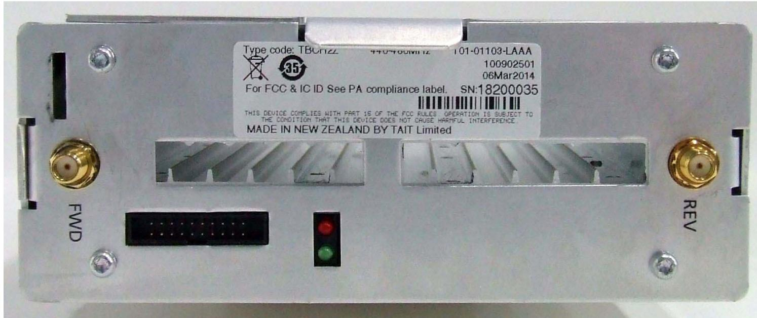
Photograph 09: Reciter module – Front panel
