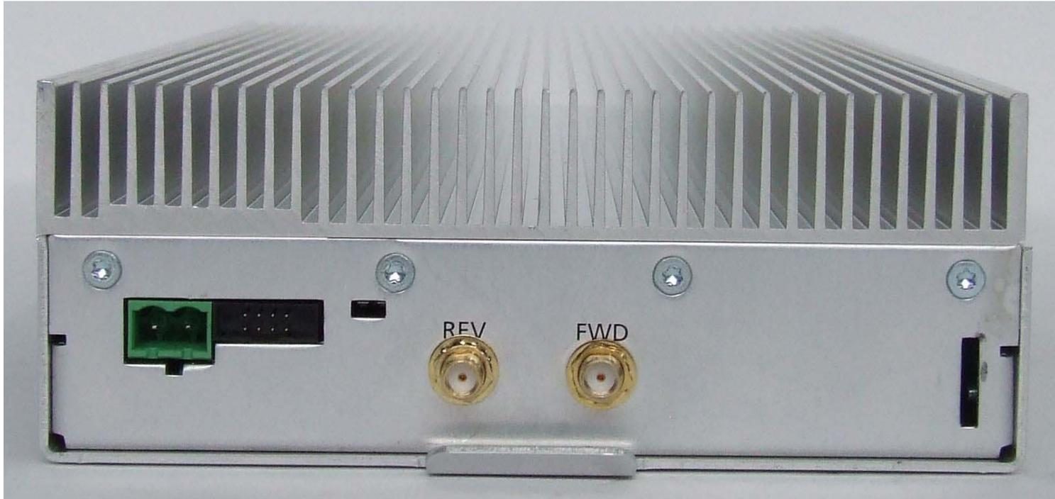
Photograph 07: PA module – Front panel
