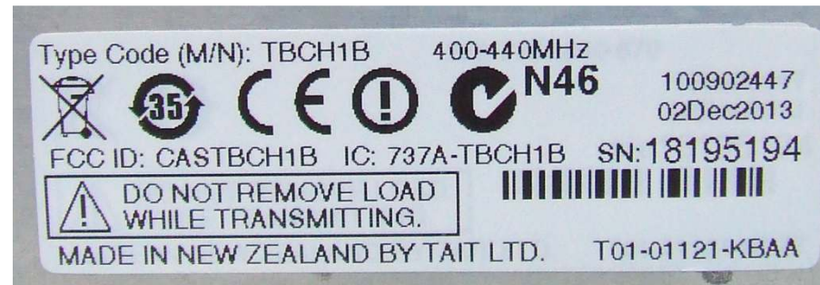
Photograph 03: 100W PA module – Compliance label
