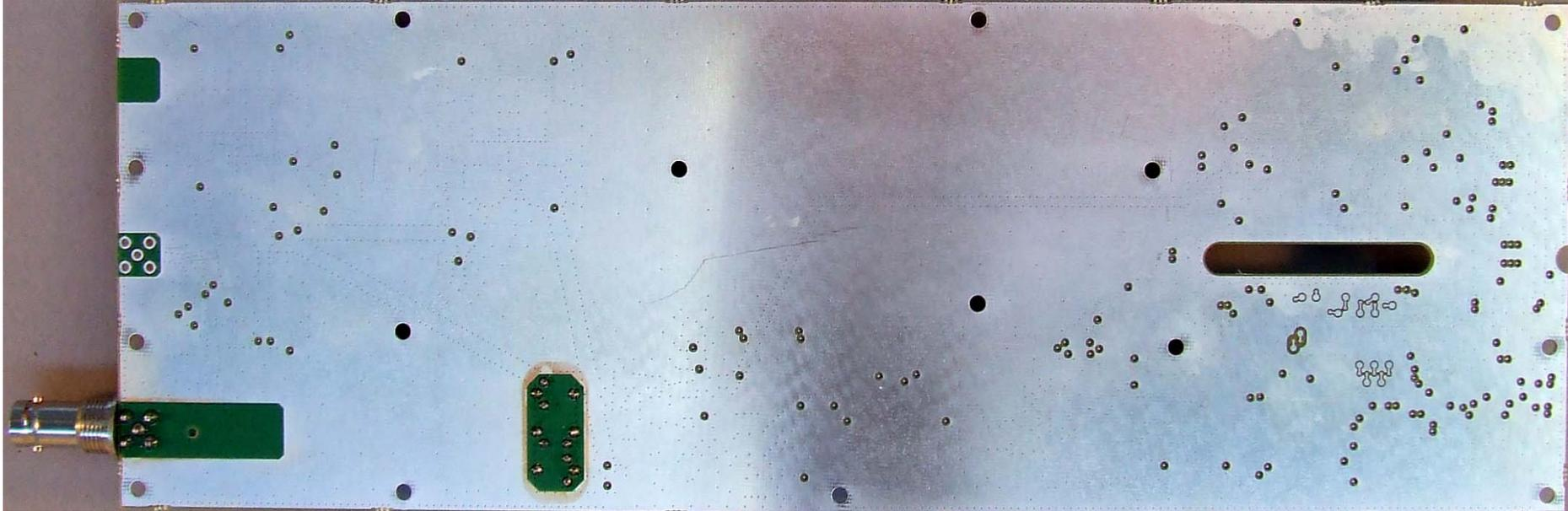
Photograph 17: Reciter Receiver PCB – Bottom
