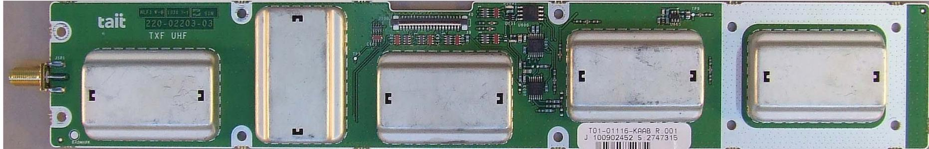
Photograph 18: Reciter TXF PCB – Top (with shields)
