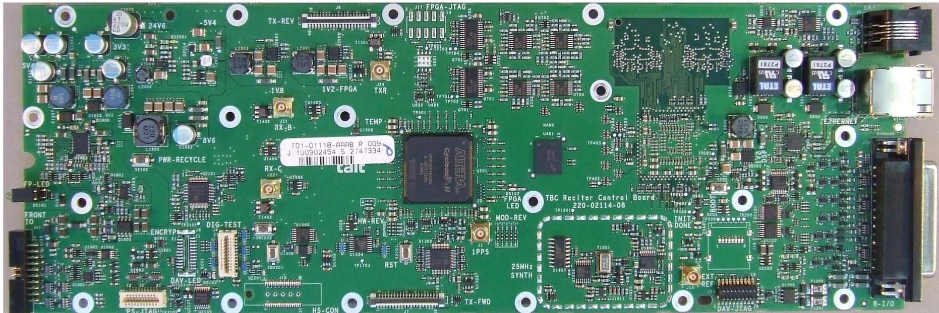
Photograph 13: Reciter Control PCB – Top (without shields)
