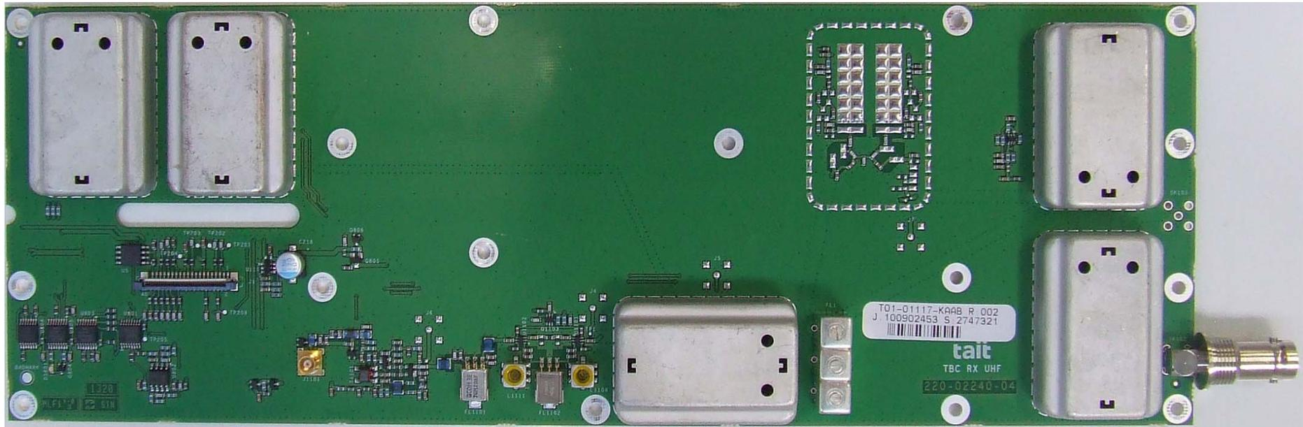
Photograph 15: Reciter Receiver PCB – Top (with shields)
