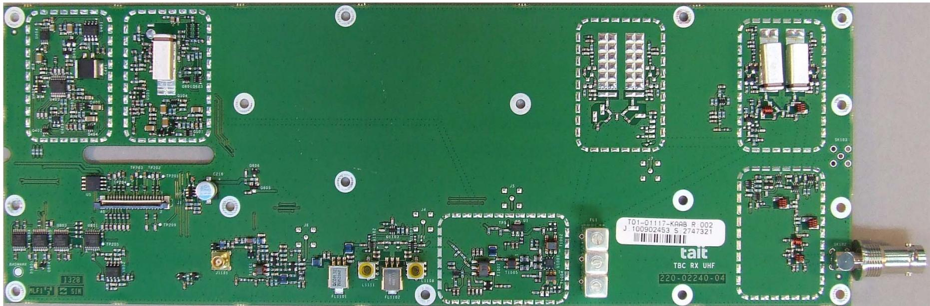
Photograph 16: Reciter Receiver PCB – Top (without shields)
