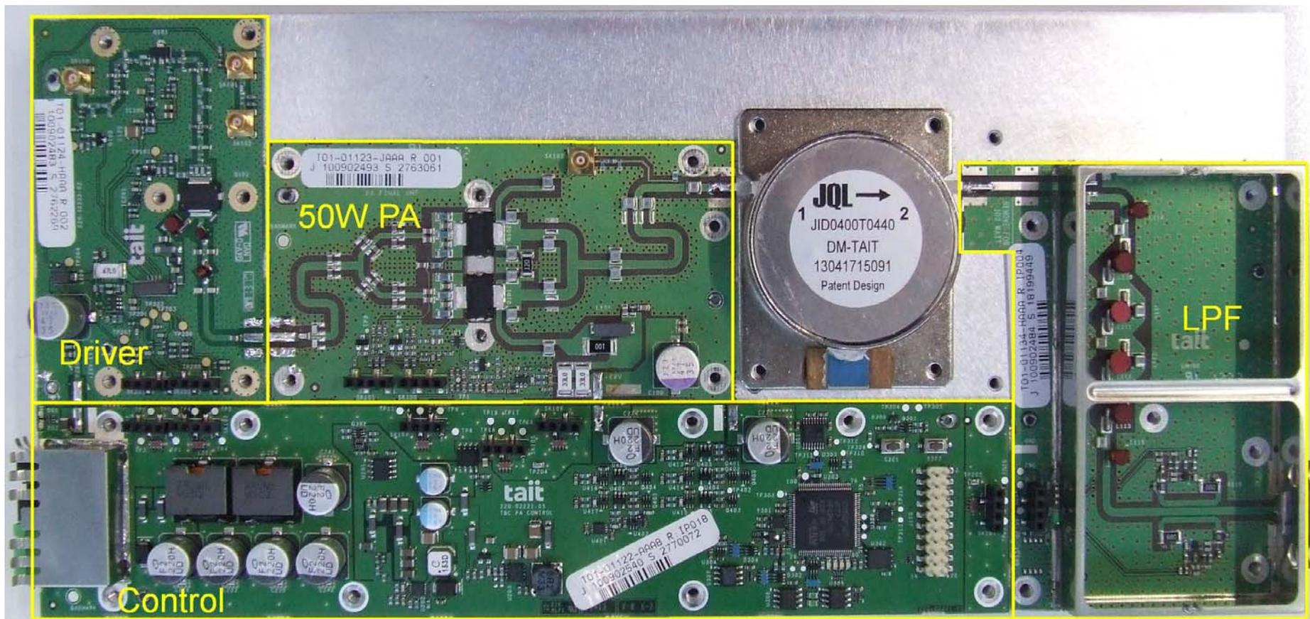
Photograph 01: 50W PA module – Internal view
