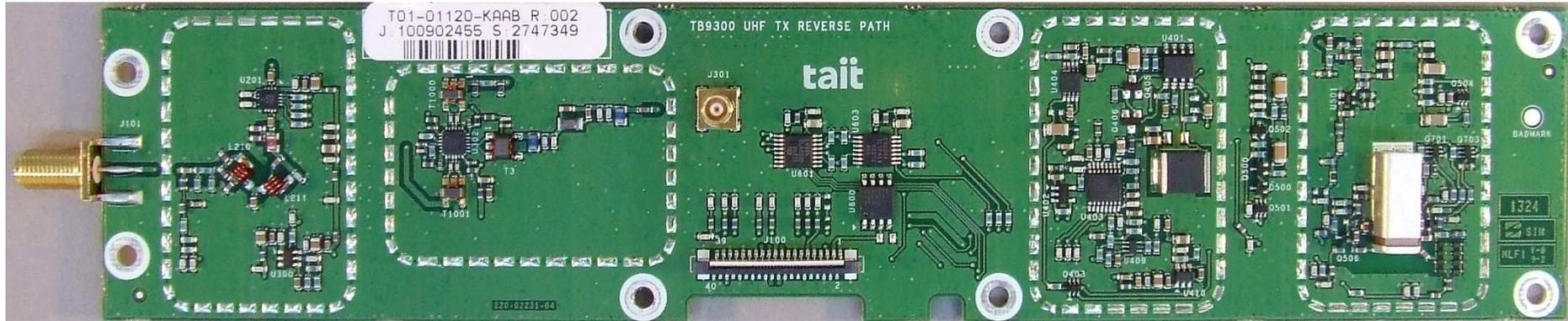
Photograph 22: Reciter TXR PCB – Top (without shields)
