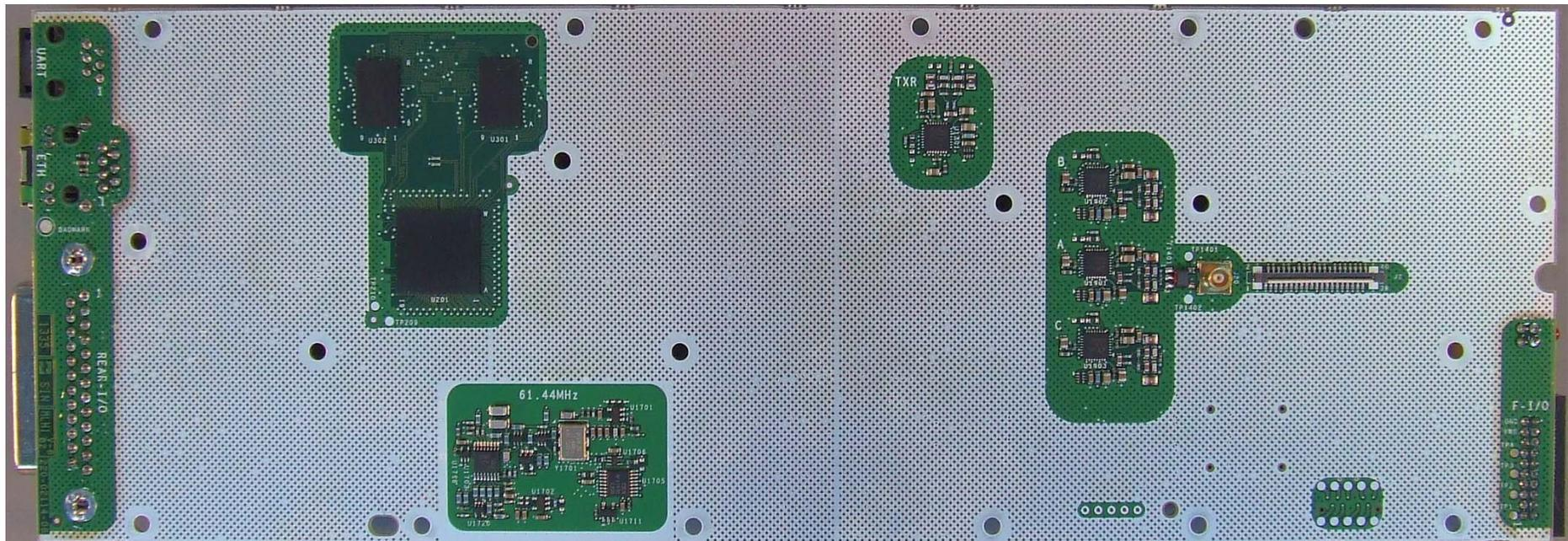
Photograph 14: Reciter Control PCB – Bottom
