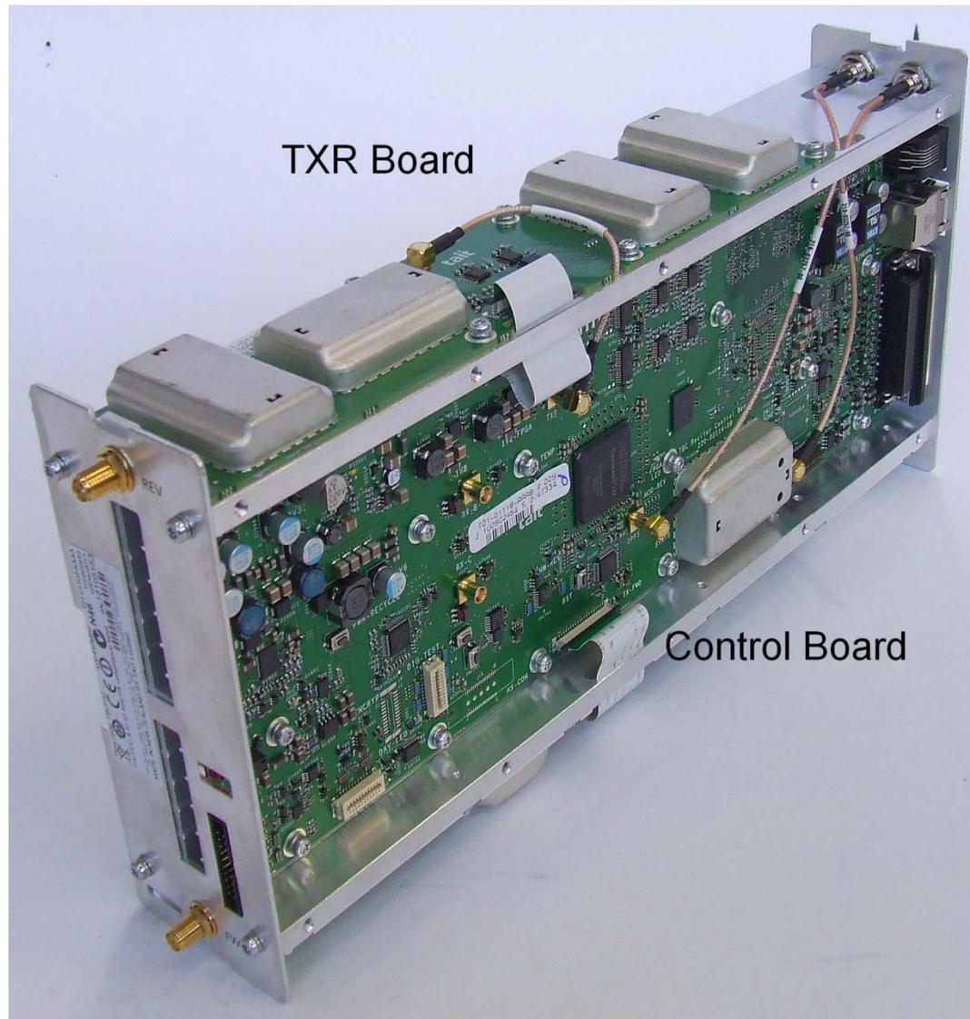
Photograph 11: Reciter module – Internal (Control PCB side)
