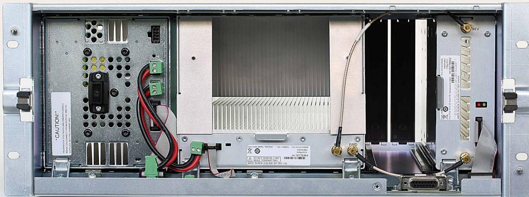
TBCB1B External Subrack Front (with front panel removed)
