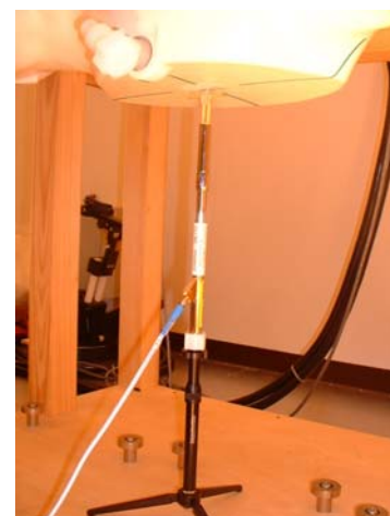
2450MHz System performance check setup
