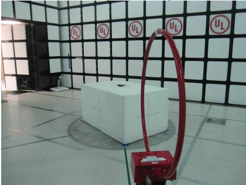
RADIATED BACK PHOTO (BELOW 30MHz)
