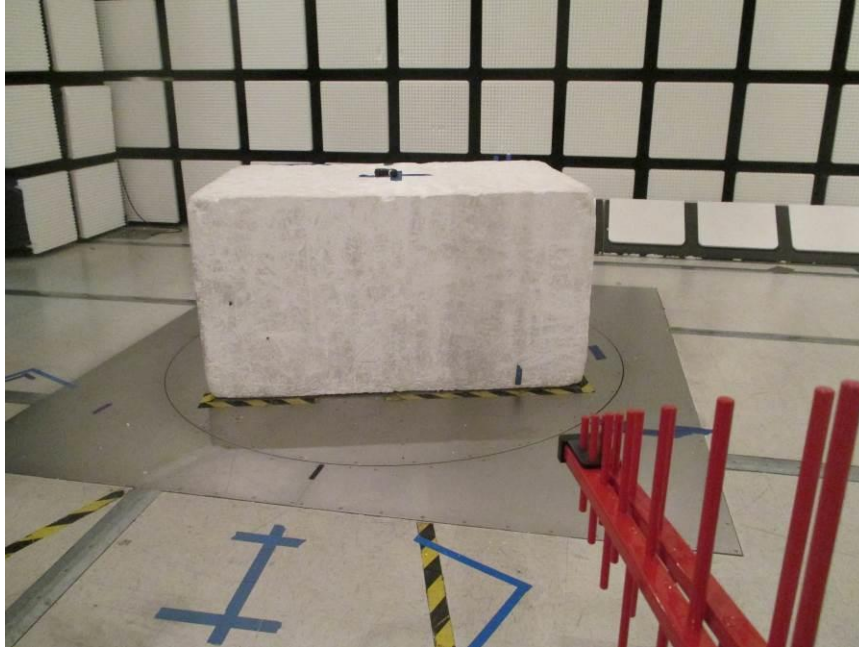
RADIATED FRONT PHOTO (BELOW 1 GHz)
