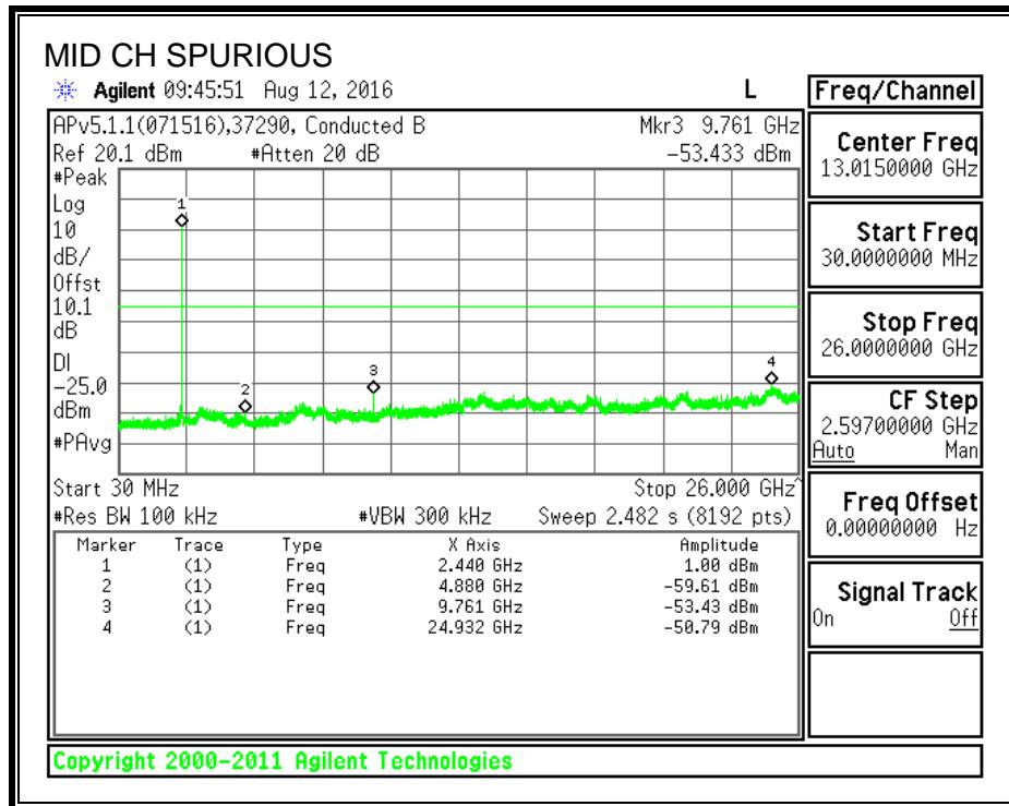
Note: Conducted spurious limit should be -17.0dBm, but compliant to lower limit of -25dBm.
