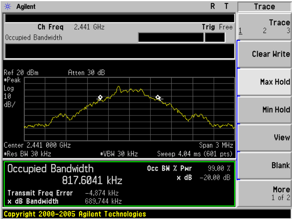
TEST PLOT OF BANDWIDTH FOR MIDDLE CHANNEL
