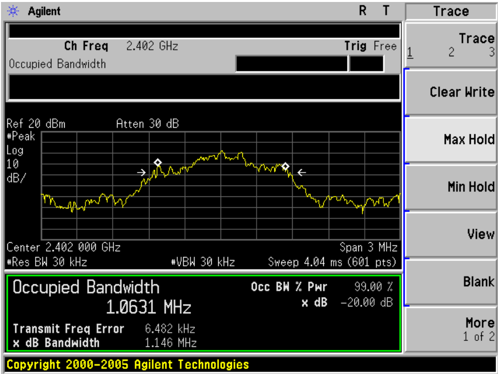
TEST PLOT OF BANDWIDTH FOR LOW CHANNEL
