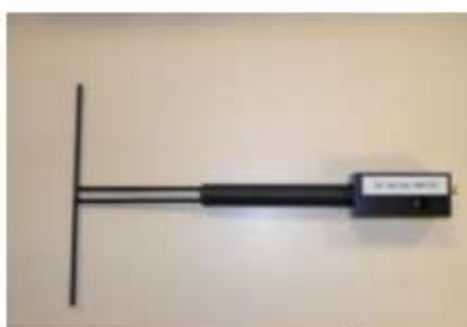
Figure 1 – Satimo COMOSAR Validation Dipole
