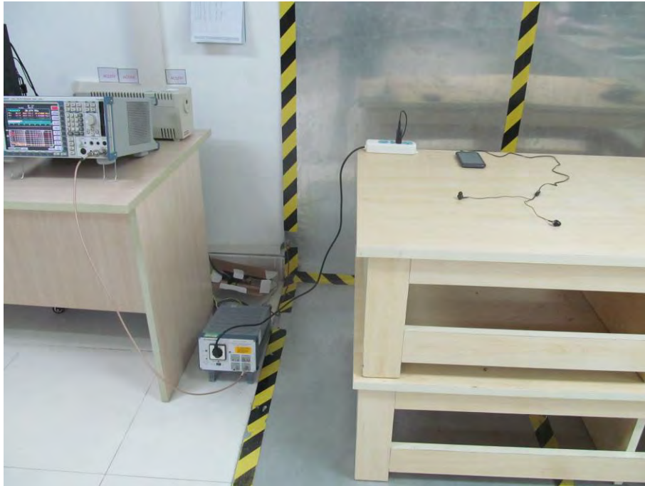
FCC RADIATED EMISSION TEST SETUP
