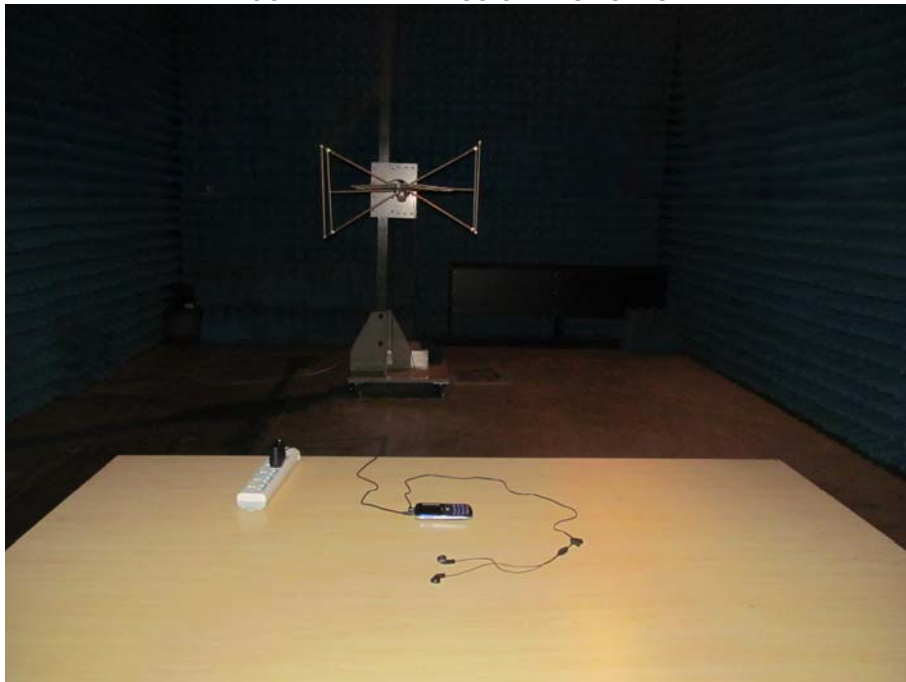
FCC RADIATED EMISSION TEST SETUP
