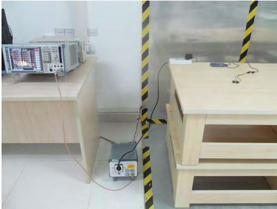
FCC RADIATED EMISSION TEST SETUP
