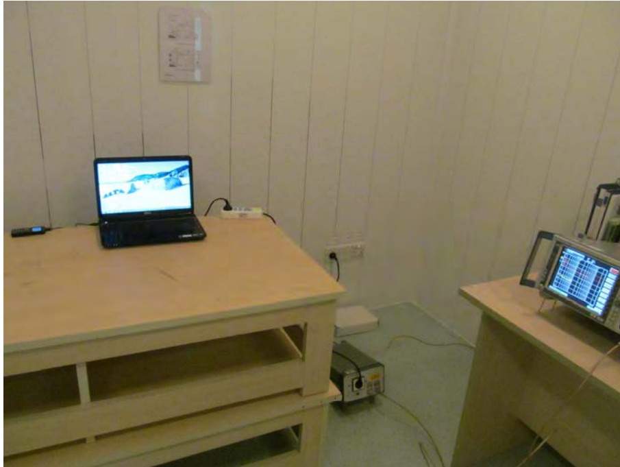
FCC RADIATED EMISSION TEST SETUP
