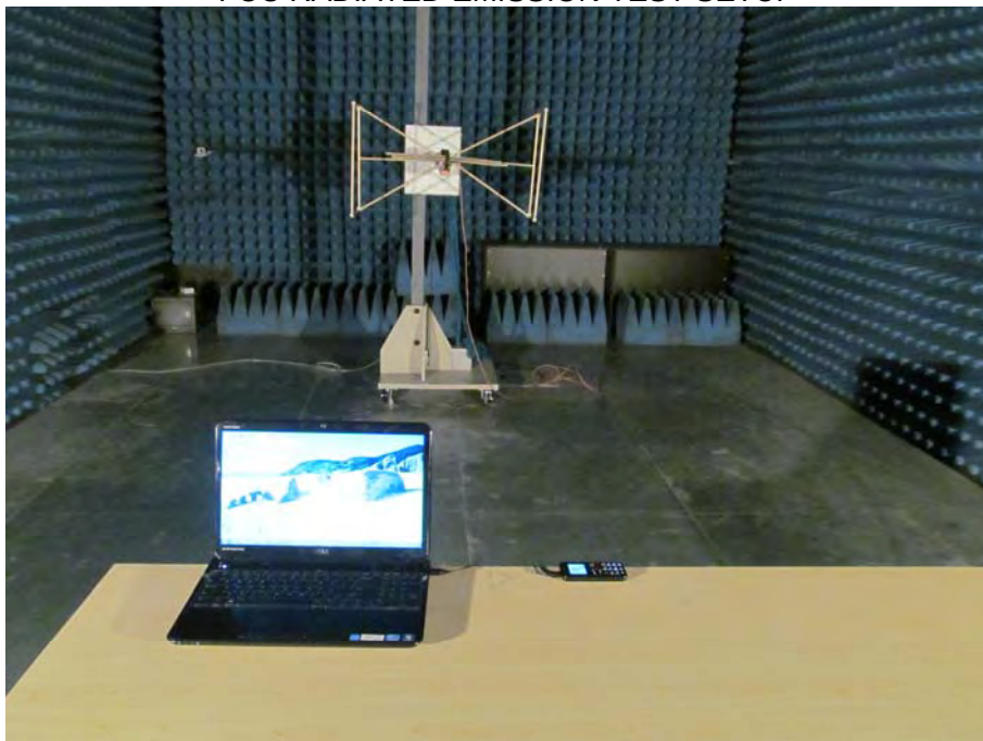
FCC RADIATED EMISSION TEST SETUP
