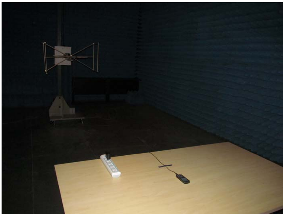
FCC RADIATED EMISSION TEST SETUP
