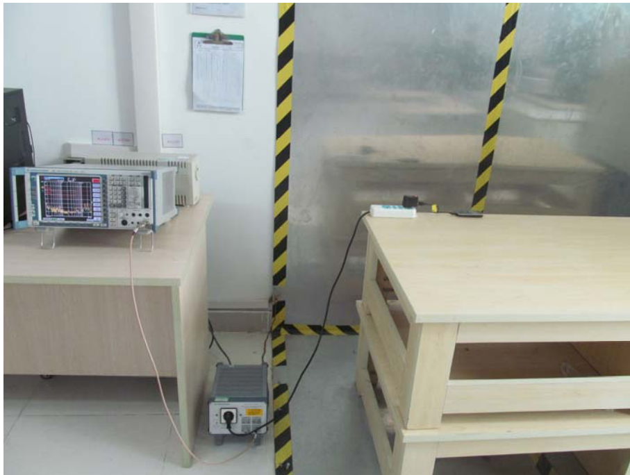
FCC LINE CONDUCTED EMISSION TEST SETUP
