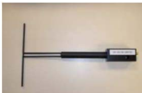
Figure 1 – Satimo COMOSAR Validation Dipole
