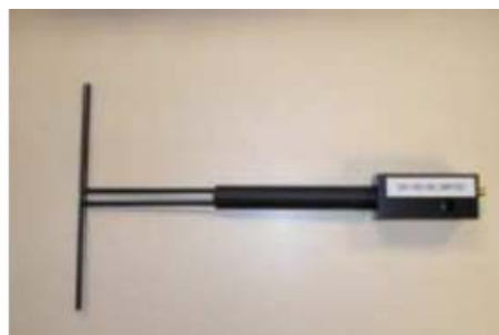
Figure 1 – Satimo COMOSAR Validation Dipole
