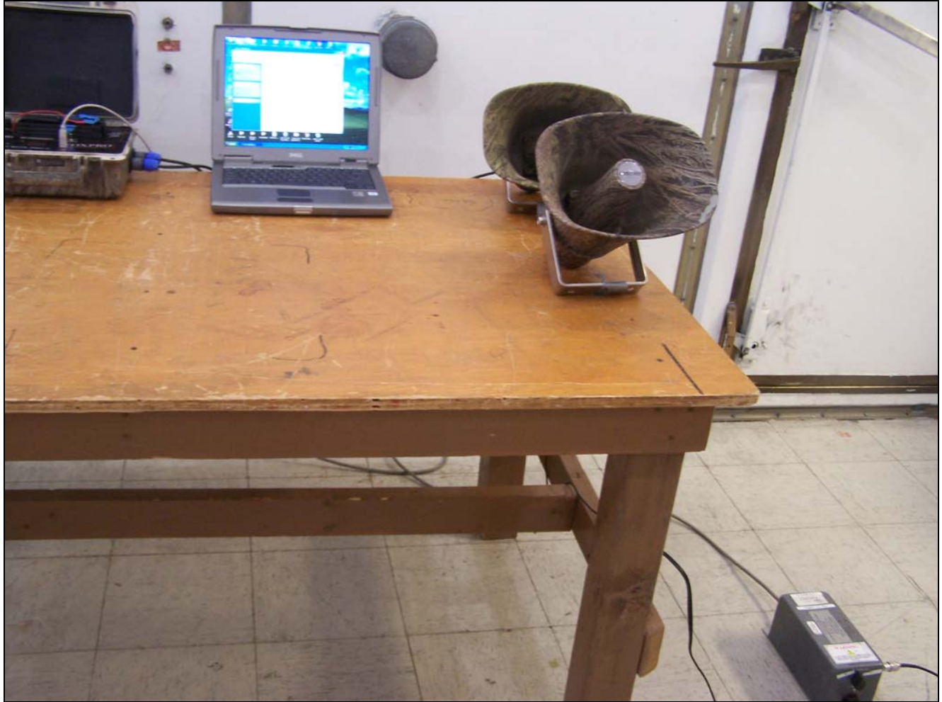
Photograph 2. Conducted Emissions, Test Setup
