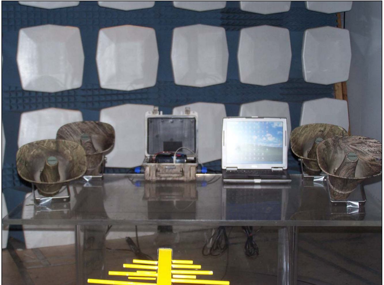
Photograph 3. Radiated Emissions, Test Setup
