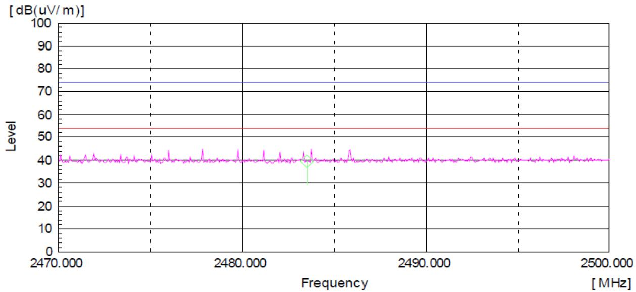
AV Detector: RBW: 1MHz, VBW: 10 Hz (2 470.0 MHz - 2 500.0 MHz), Worst case (High, Vertical)
