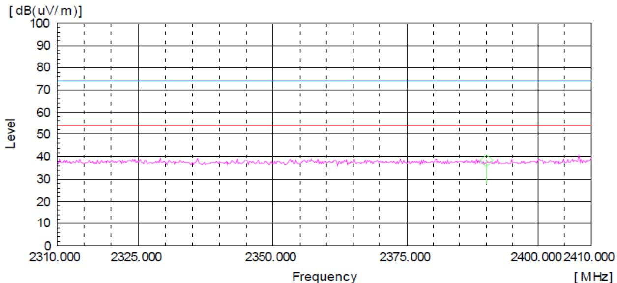
AV Detector: RBW: 1 MHz, VBW: 10 Hz (2 310 MHz - 2 410 MHz), Worst case (Low, Vertical)
