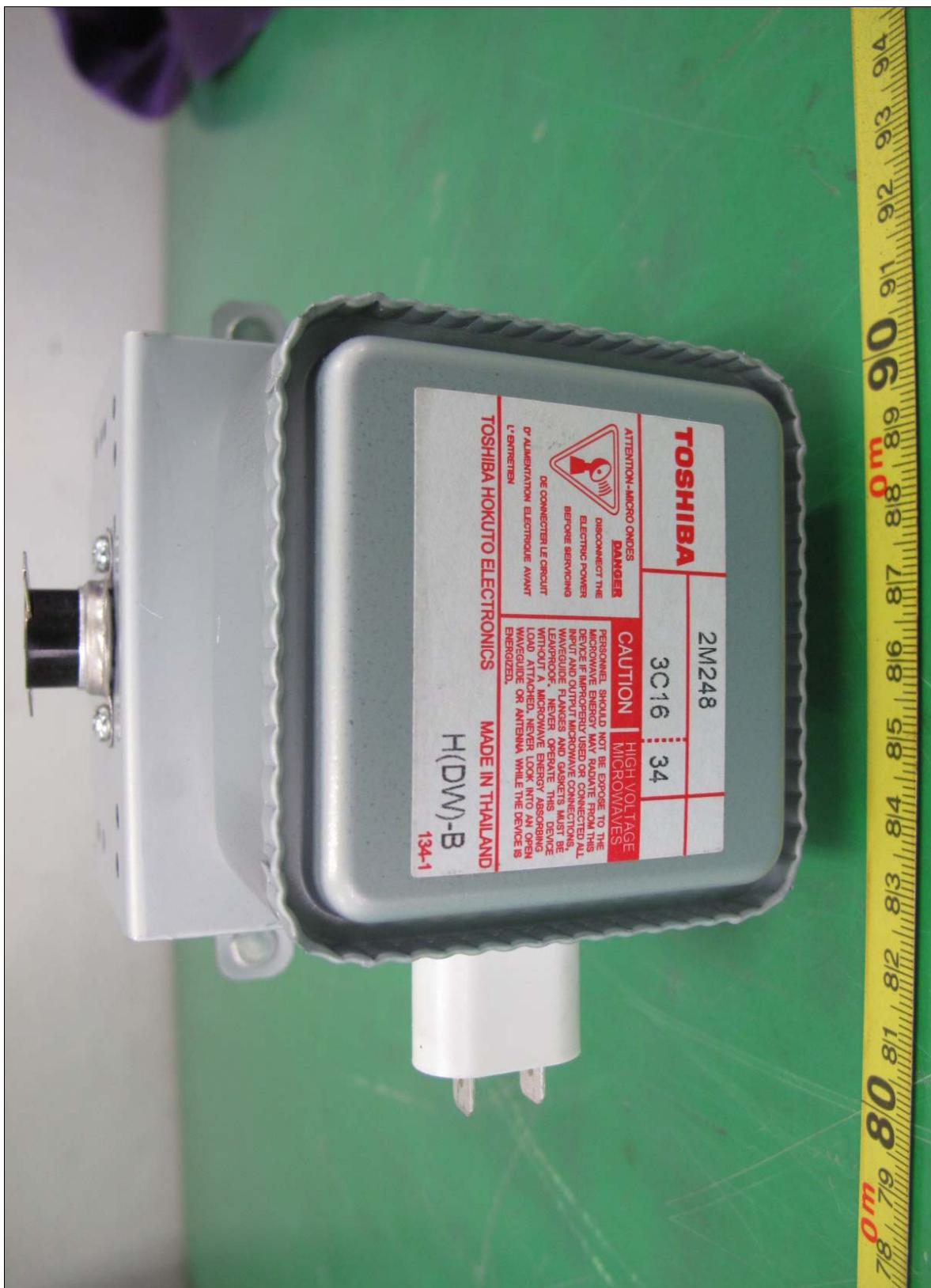
● Rear View of Magnetron
