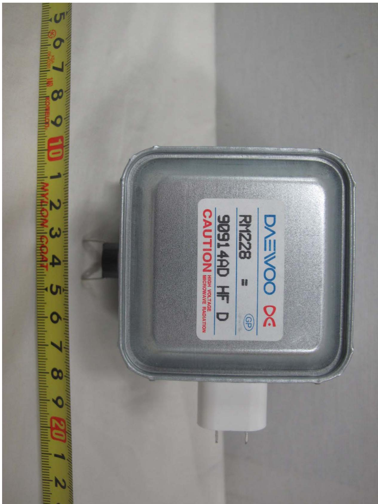
● **Rear View of Magnetron**
