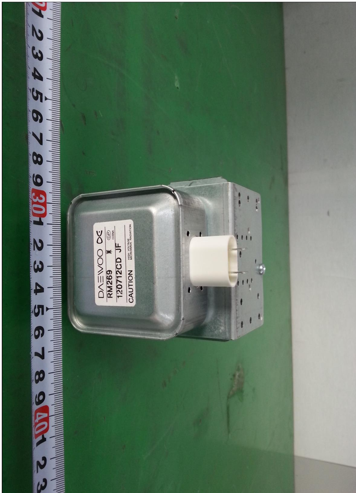
● **Rear View of Magnetron**
