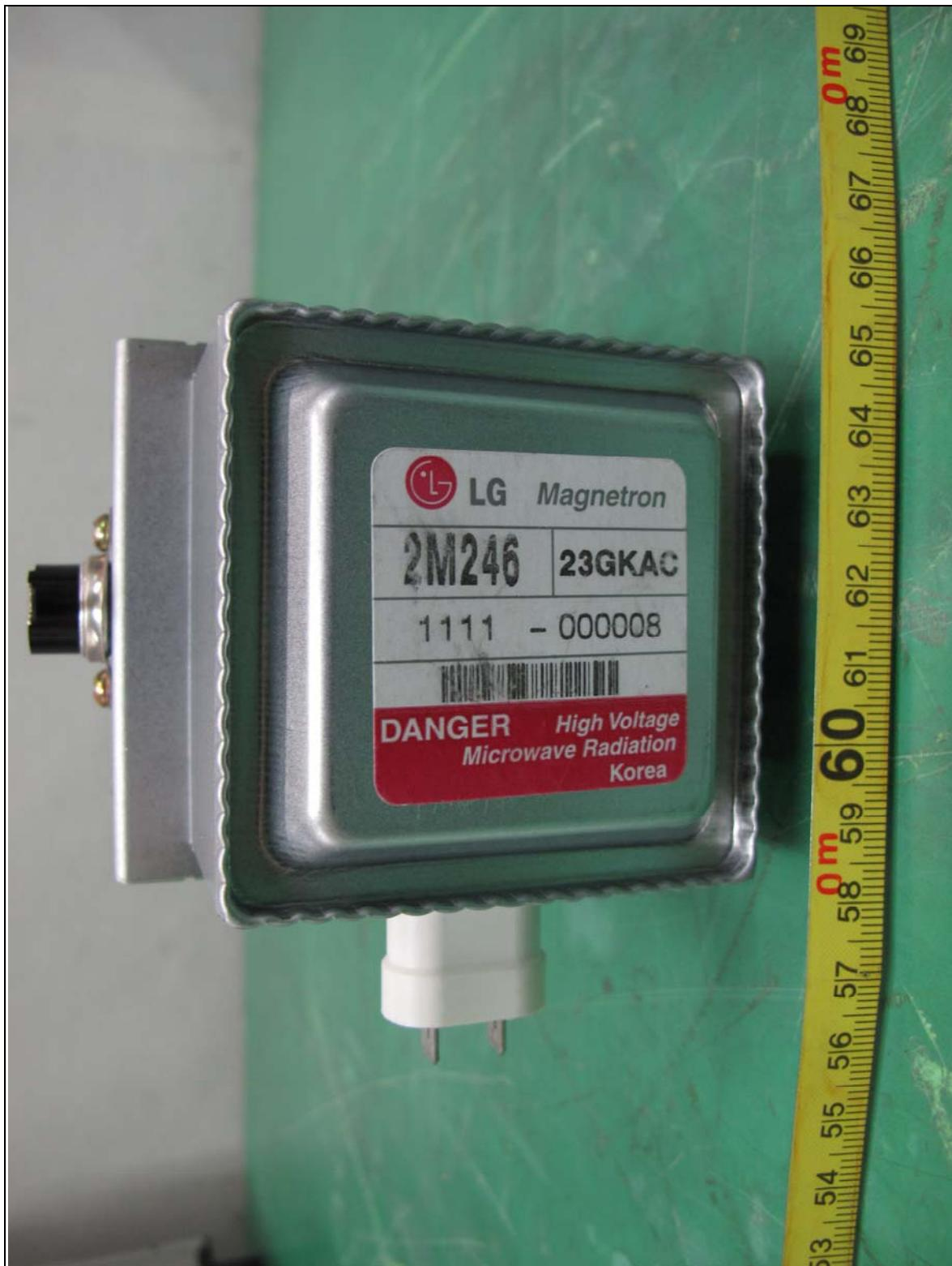
● **Rear View of Magnetron**
