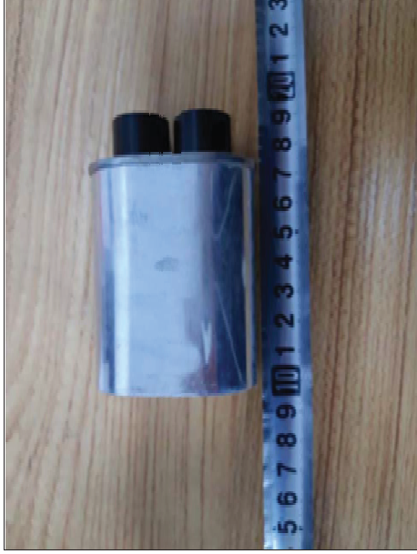
17. Rear View of H.V. CAPACITOR
