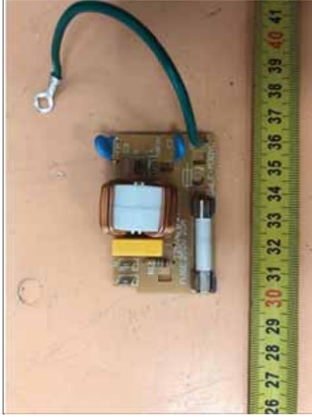
18. Front View of Noise Filter
