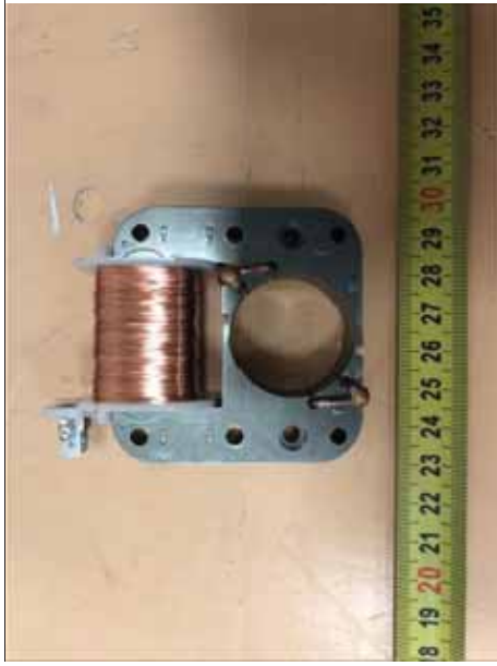
10. Front View of FAN MOTOR
