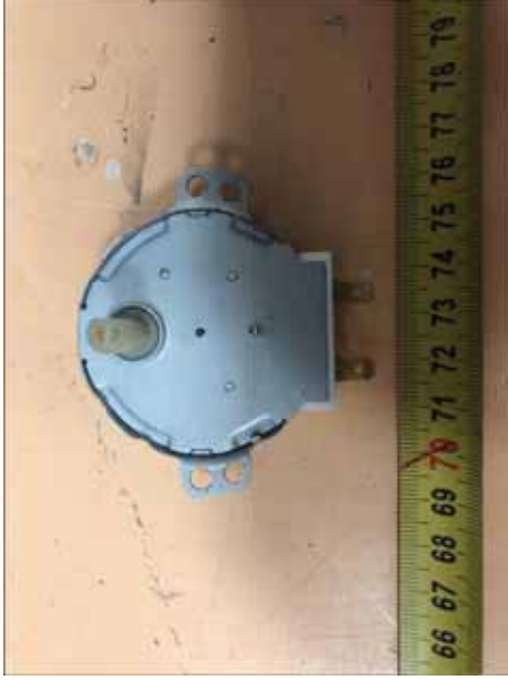
9. Rear View of Synchronous Motor
