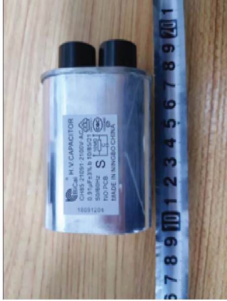
16. Front View of H.V. CAPACITOR
