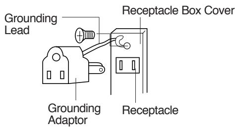
“THE CANADIAN ELECTRICAL CODE DOES NOT ALLOW THE USE OF THE GROUNDING ADAPTOR”
