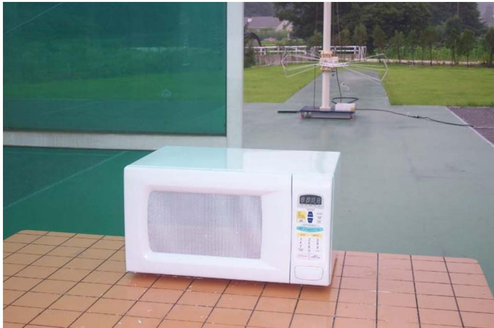
● Radiated Test Picture – 30MHz ~ 1GHz (Rear)
