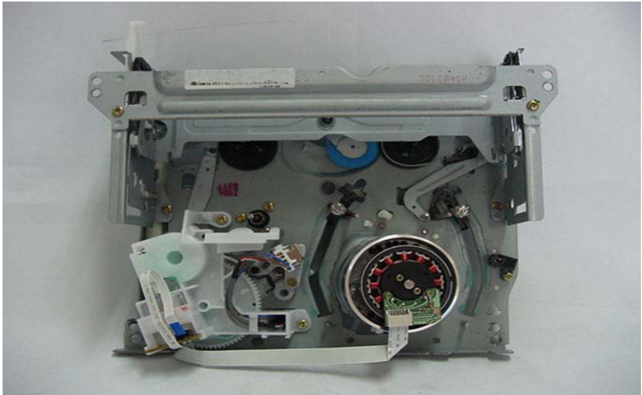
VCR Deck Top View
