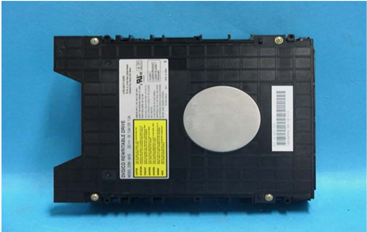
DVD Deck Top View (Removed Cover)
