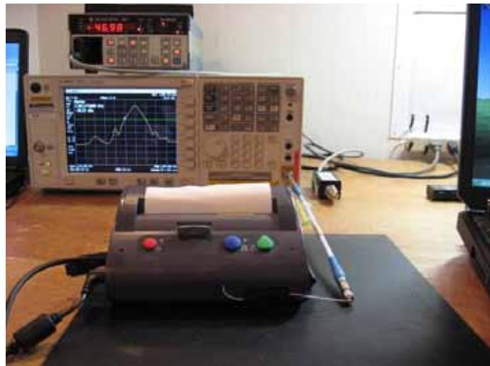
***Transmitter Radiated Spurious Emissions (RF Radiated test)***
