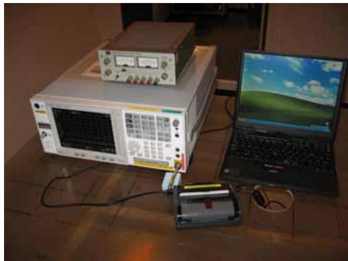
***Transmitter Radiated Spurious Emissions (RF Radiated test)***
