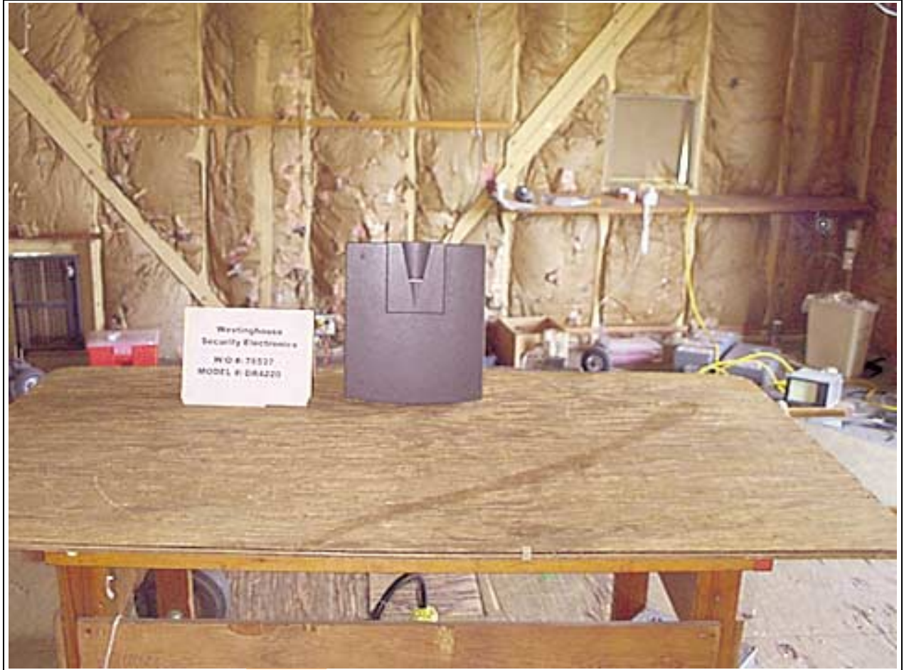
Radiated Emissions - Front View
