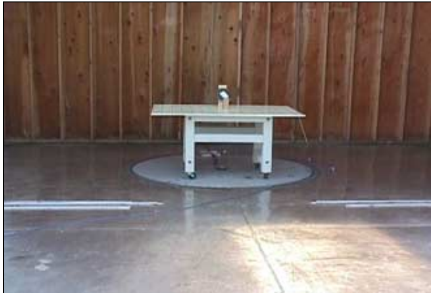
View of the EUT during Radiated Emission Testing on the 10 Meter OATS
