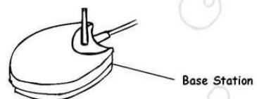
Be sure to use a standard 9V DC 300mA center positive +--- AC adapter to power the base station. Always plug the adapter into the base station before plugging it into the mains. Always make sure that the unit is off before connecting a power supply to the unit.
