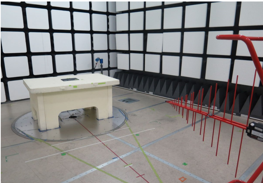
Figure 8 Radiated Spurious Emissions Test Setup (30MHz-1GHz) – BTLE X orientation.
