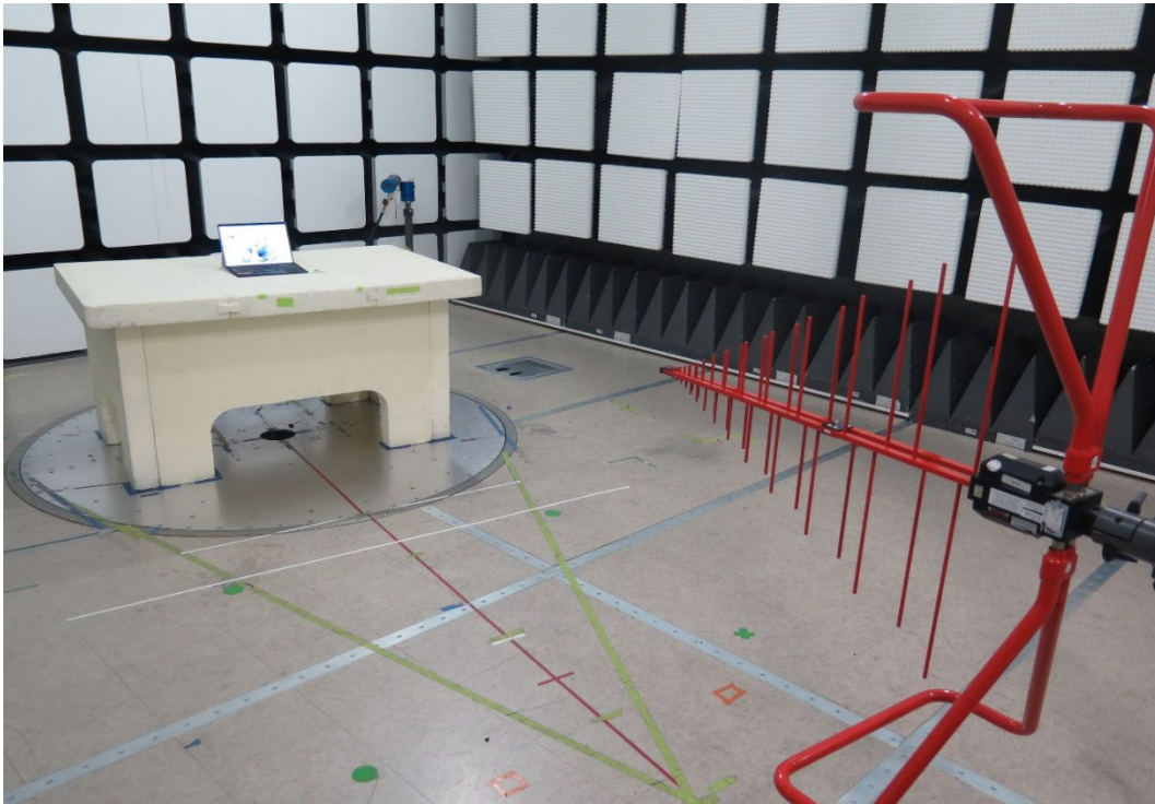
Figure 7 Radiated Spurious Emissions Test Setup (30MHz-1GHz) – NFC
