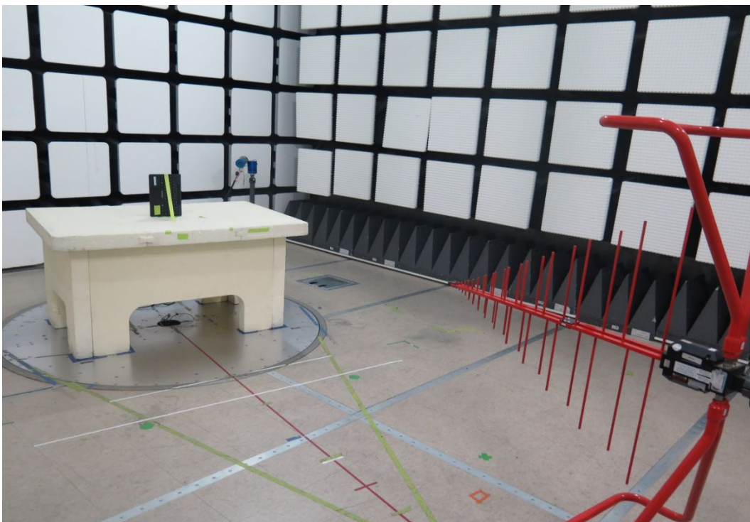
Figure 10 Radiated Spurious Emissions Test Setup (30MHz-1GHz) – BTLE Z orientation
