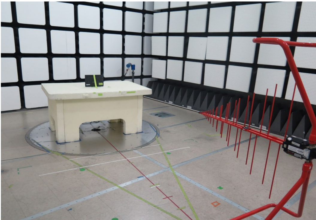
Figure 9 Radiated Spurious Emissions Test Setup (30MHz-1GHz) – BTLE Y orientation
