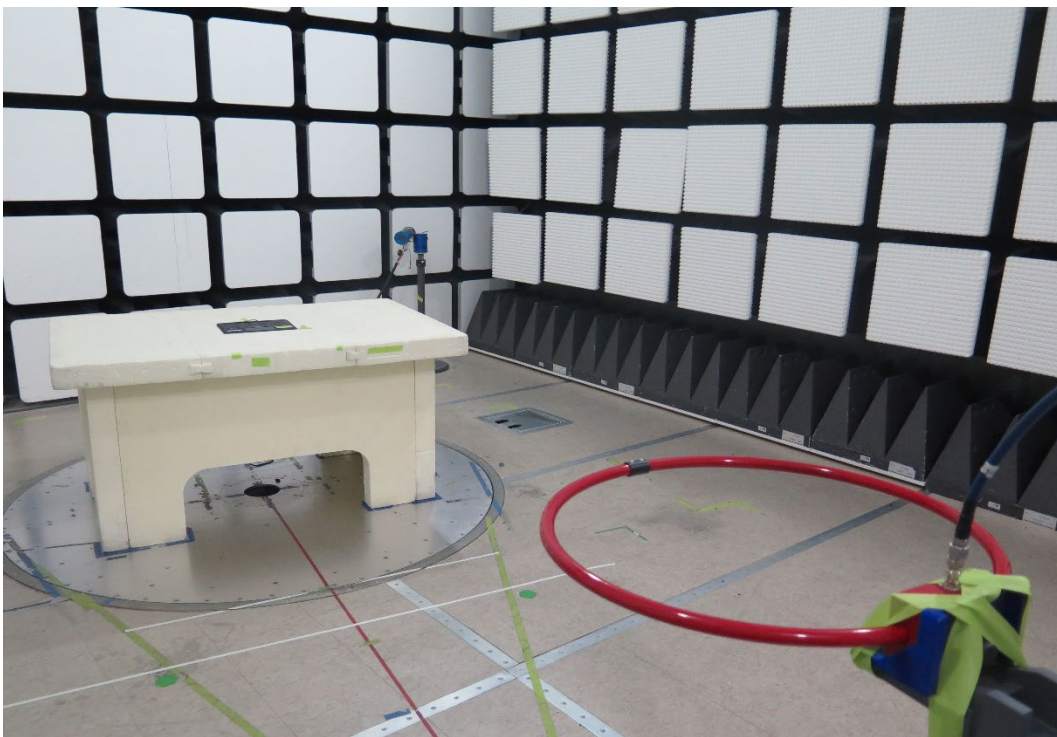
Figure 6 Radiated Spurious Emissions Test Setup (9KHz-30MHz) Loop ground parallel orientation – BTLE
