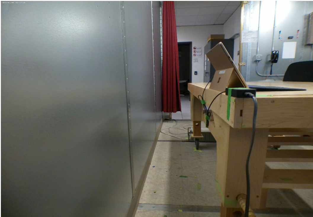
Figure 16 AC Line Conducted Emissions Test Setup - Side View
