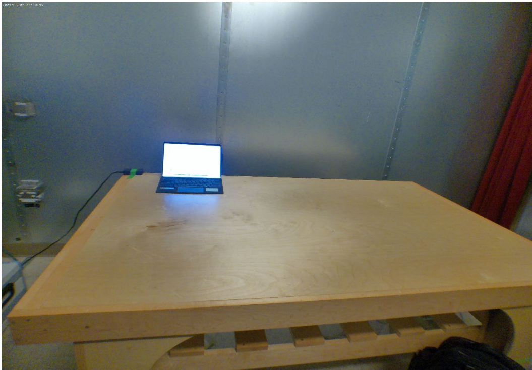
Figure 14 AC Line Conducted Emissions Test Setup - Front View
