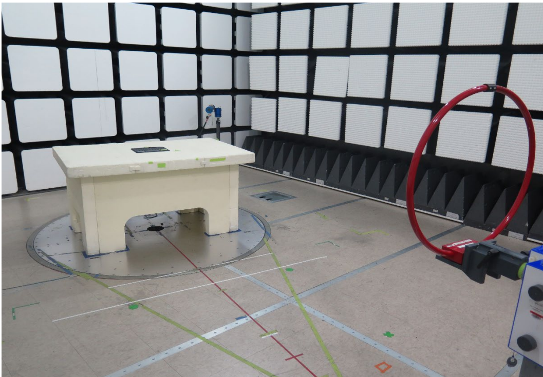
Figure 4 Radiated Spurious Emissions Test Setup (9KHz-30MHz) Loop parallel orientation - BTLE
