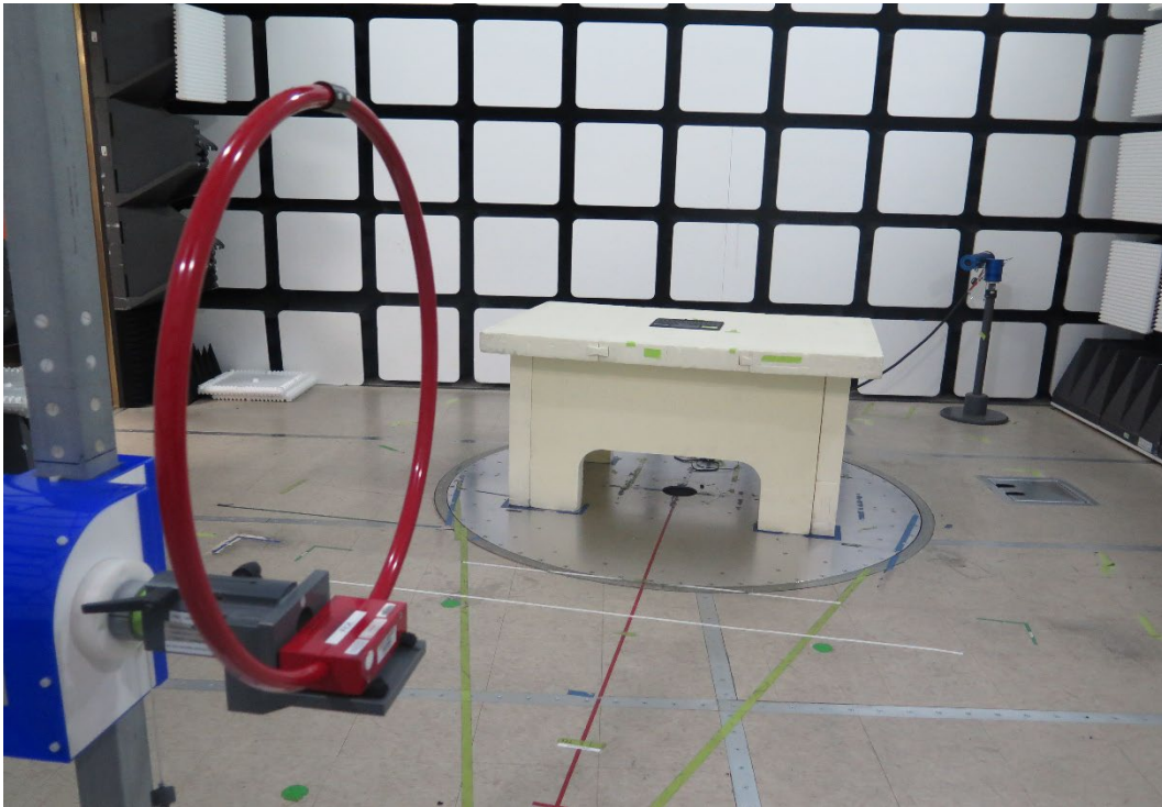
Figure 5 Radiated Spurious Emissions Test Setup (9KHz-30MHz) Loop perpendicular orientation - BTLE
