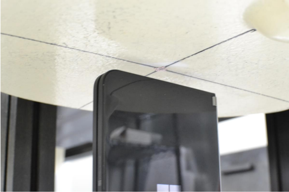
SAR Test Setup Photo 21– Closed Configuration (Handset), Hotspot, Bottom Edge, 10 mm
