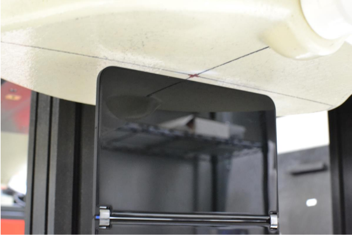
SAR Test Setup Photo 29– Read Configuration (UMPC), UMPC Extremity, Left Edge, 5 mm
