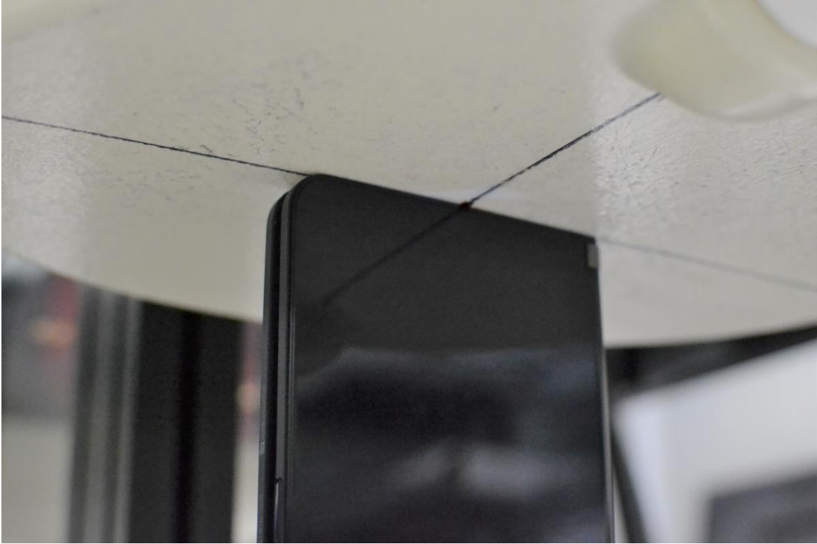
SAR Test Setup Photo 13– Flip Configuration (Handset), Phablet, Bottom Edge, 0 mm
