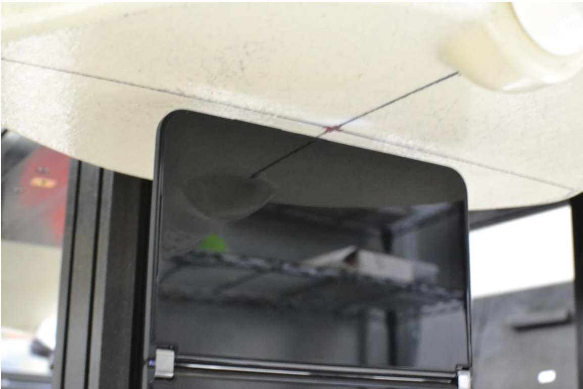
SAR Test Setup Photo 28– Read Configuration (UMPC), UMPC Body, Right Edge, 5 mm
