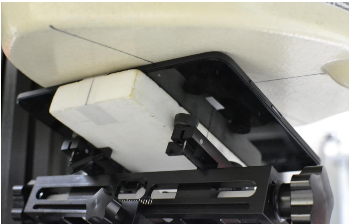
SAR Test Setup Photo 31– Flat Configuration (Body), Body, Back Side, North Antenna, 0 mm
