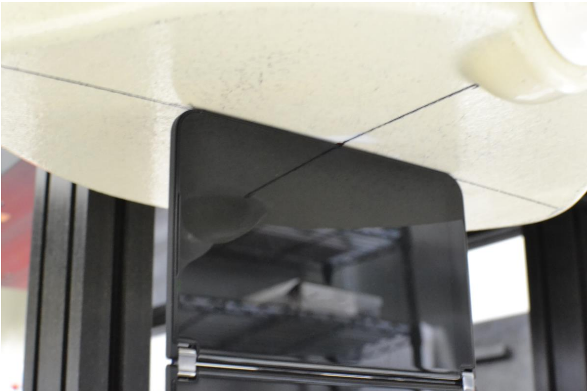
SAR Test Setup Photo 34– Flat Configuration (Body), Body, Right Edge, 0 mm
