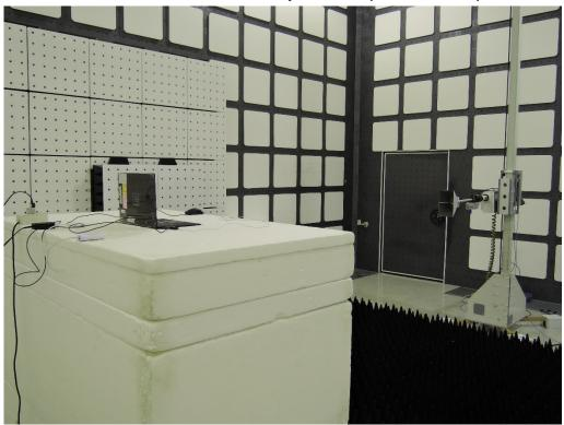
Radiated Emission Set up Photos (Above 18GHz)
