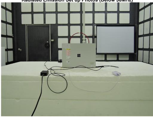
Radiated Emission Set up Photos (Below 1GHz)
