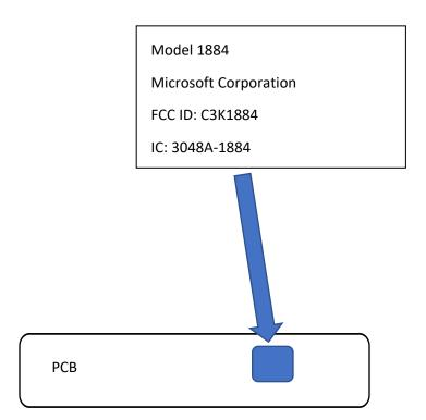
Label located on radio module shield top of EUT
