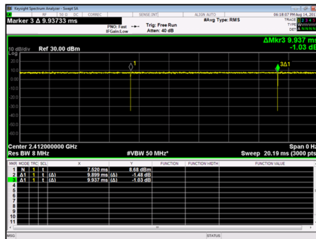
Figure 9-5. Duty Cycle 802.11n -Path A
