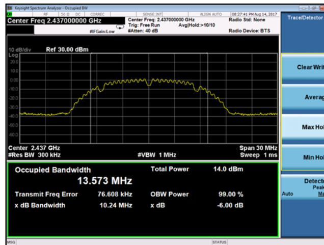
Plot 9-44 Chain A 99% Bandwidth 802.11b - Ch.6 (2437 MHz)
