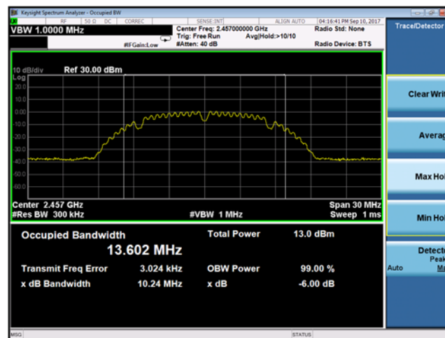
Plot 9-45 Chain A 99% Bandwidth 802.11b - Ch.10 (2457 MHz)
