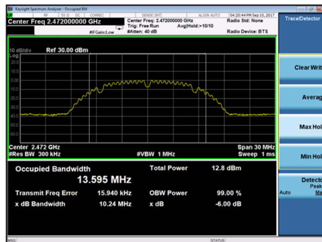
Plot 9-48 Chain A 99% Bandwidth 802.11b - Ch.13 (2472 MHz)
