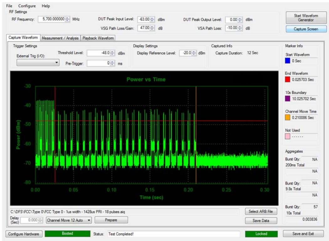
Figure 8. Channel Closing Time - Ch. 140 (5700 MHz)
