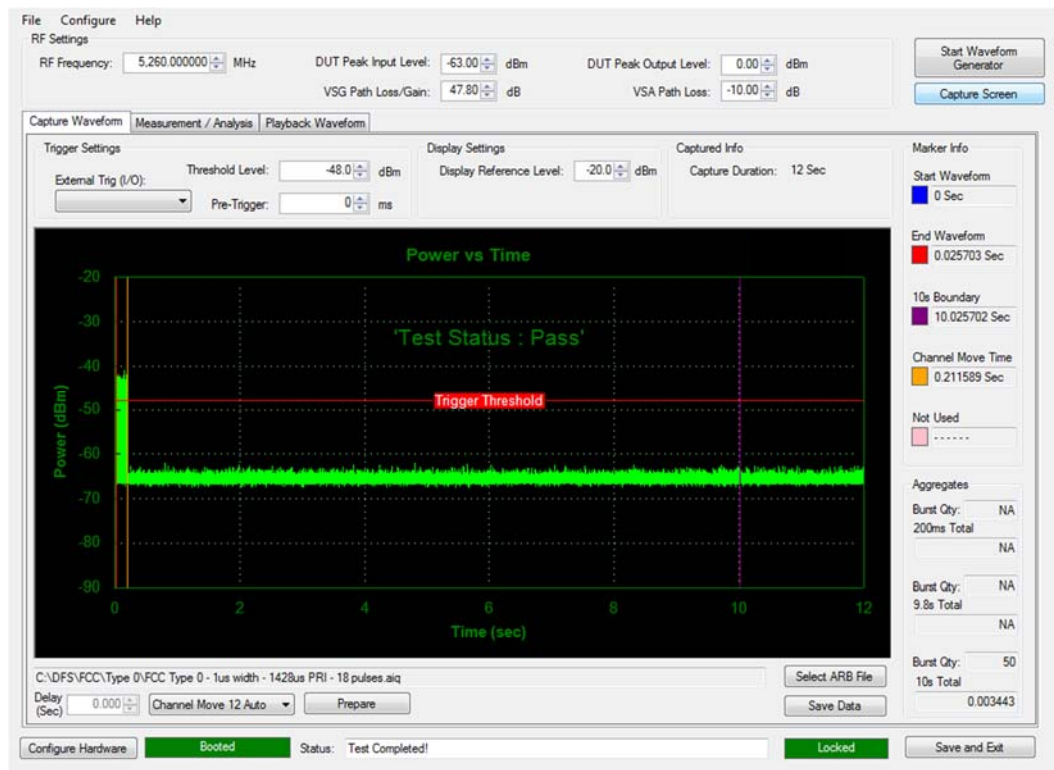
Figure 5. Channel Move Time 10s – Ch. 52 (5260 MHz)
