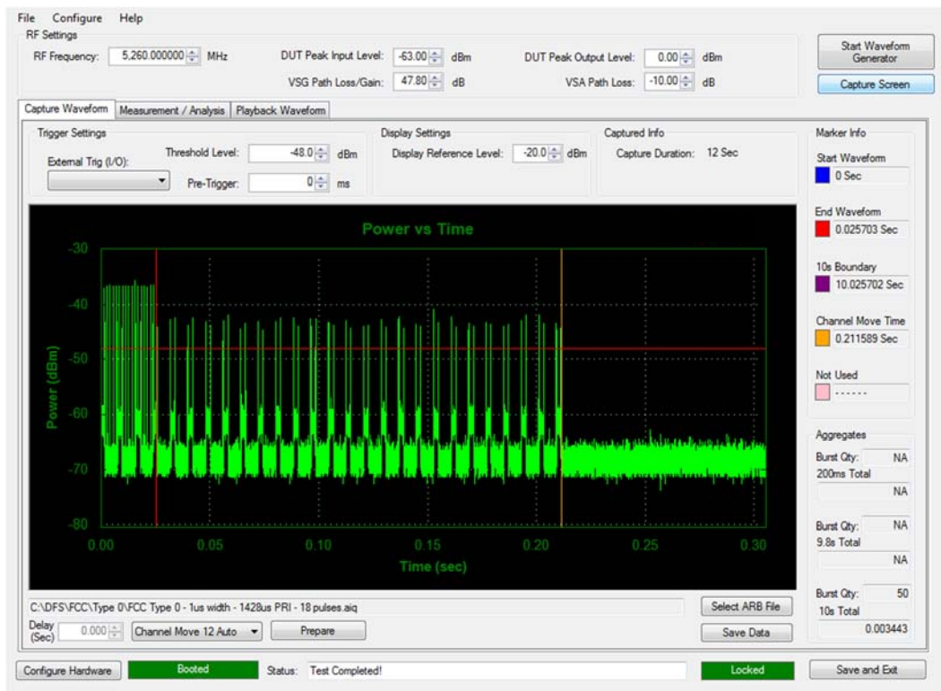
Figure 7. Channel Closing Time - Ch. 52 (5260 MHz)
